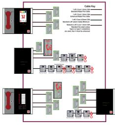
The Lexicomm ViLX-TMS is a self contained enclosure housing a master handset, 4.3" touch screen, one to four dual line cards, an EN54-4:A2 2006 power supply & battery charger and can be surface or flush mounted (Using the ViLX-CBZ Bezel).
