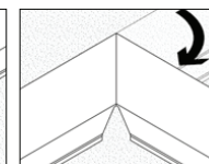
STEP 2 - Make a single cut on the opposing side shoulder (see step 1 diagram) then bend in the corner.
