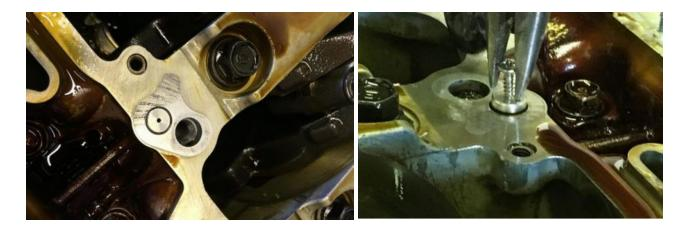
You can use a small drill bit to catch the inside of the plug, or drill it first and twist in a small machine screw. If it doesn't pull out on the end of the drill bit, you can use pliers to remove it.
