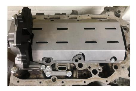
Once bolted down, install the oil jet plug as shown:
