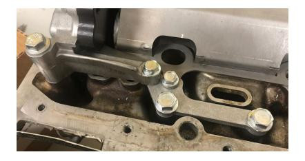
If you are installing this in a Miata, you'll want to remove the stock pickup side of the oil pump and install the KMiata Type S oil pump adapter.
