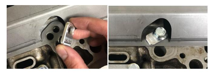
If applicable, the KMiata oil pickup tube can now be installed.
