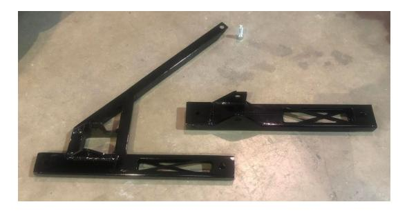
They both install in the exact same manner, with the exception of the third mounting point that's required on the NA8 brace. Since the M12 holes for the OEM subframe brace protrude forward 2 inches on the NA8 subframe, a third mounting point is necessary.
