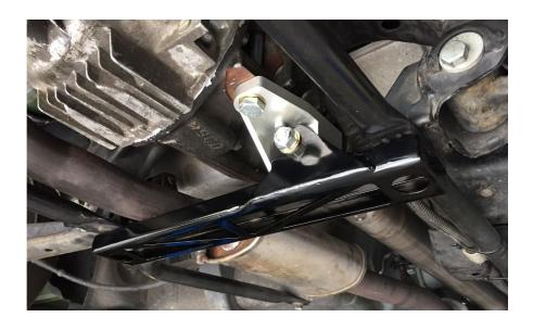
If the brace is not installed, the pinion angle will not be correct and the mounting points on the subframe will gradually fatigue and may eventually crack.
