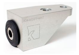
This mount bolts to the diff housing with the supplied 120mm and 130mm long bolts. The small aluminum figure eight shaped piece found on top of the diff is retained. The front bolt threads into the aluminum mount from the top of the diff, and the rear bolt is inserted from the bottom and secured from the top of the diff with the supplied locking nut and washer.
