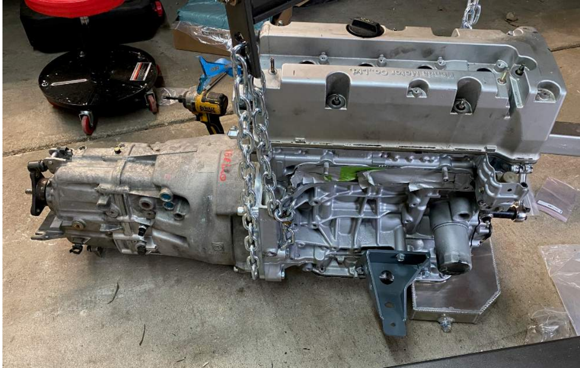
Engine mount arms can also be bolted to the block at this time.
