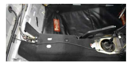
The wire can also be routed through the factory grommet.
