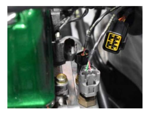
If you're swapping an NA, you will need to source the three pin ECT sensor from an NB.
