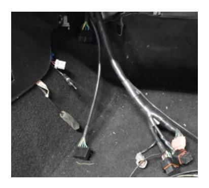
The Haltech ECU can be mounted in a variety of places under the dash depending on your preferences and usage for the car. For a street car, we prefer to mount it in the glove box or in the passenger air bag tray (assuming the airbag is deleted). A USB cable can stay plugged in and rolled up in the glove box as well.
