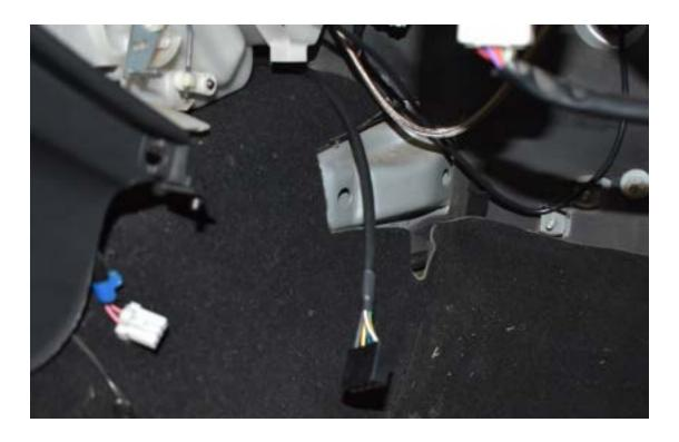
The remaining portion of the harness will still be hanging out of the gauge cluster opening.
