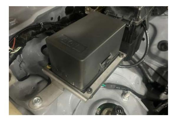
As you can see in this photo, the fuse box is supplied with constant 12V power thanks to the black wire and eyelet that extends out of the box. Connect this wire directly to the main fuse under the OEM fuse box. Remove the bolt that secures it and tighten it back down with the eyelet below it.
