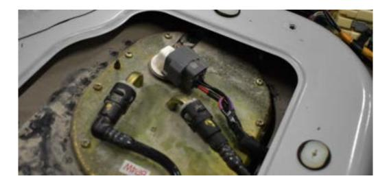
Once all of the connections have been made on the cabin harness, the rest of the installation is plug and play. Thanks to this subharness, the engine harness does not need to be permanently attached to the car and can be removed for future service.
