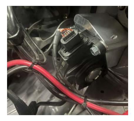
If you are using a cable throttle body, your harness does not have this connector.
