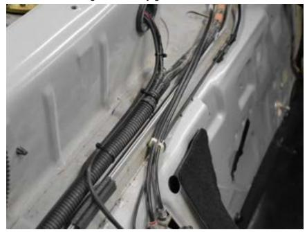
Unplug the main gray connector to the fuel pump, depin the stock wire and terminal, and replace it with the new wire and terminal. The stock fuel pump wire can be taped out of the way (red/blue in this picture).
