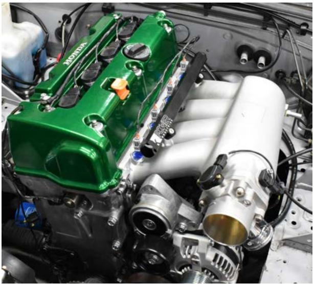
A fan relay is built into the harness as well. We recommend routing this long two wire connector around the driver side of the engine bay and connecting it directly to the OEM fan. In this picture, the IAT (intake air temp) sensor can also be seen. Regardless of intake setup, drill a hole in your piping and use a universal grommet to mount any 2002-2008 K series IAT into the pipe.
