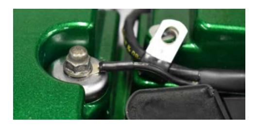
Both the K series ECT (engine coolant temp) and Miata ECT (for the stock gauge) thread into the right side exit water neck, and plug in like this:
