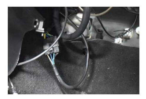
If you're using the Haltech CAN wideband and controller, it can also be connected to the ECU and the engine harness at this time with the gray 4 pin Deutsch connectors.
