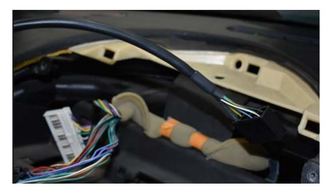
Pull the connector behind the heater core and over to the passenger side of the cabin.
