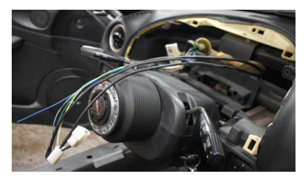
With the lower dash drop panel removed, feed the fuse adder over to the dash fuse box on the far left side of the lower dash.
