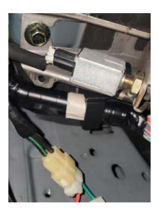
The clutch wire on our harness needs to be spliced to this switch. Again, on our NB this wire is brown/white.
