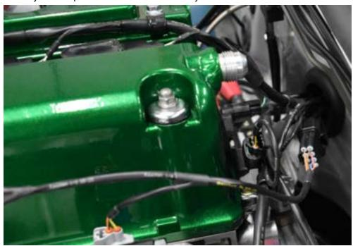
Once the subharness and remaining connectors are installed, your engine bay will begin looking like this (cable throttle body pictured):
