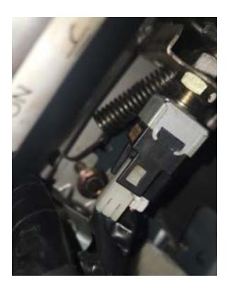
The brake wire on our harness needs to be spliced to this switch. On our NB, it is a green wire. The clutch pedal switch looks like this:
