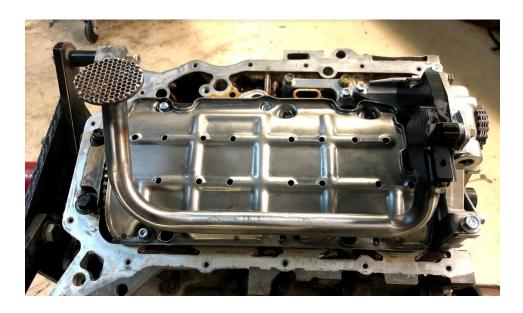
Once everything is tightened down, spin the crankshaft by hand to make sure that the connecting rods are not interfering with the tray or rails. If there is any interference, it's better to address it now before the oil pan is sealed up.
