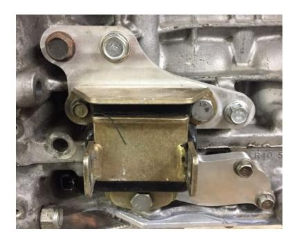
The left mount (driver side) bolts in place here, underneath the starter. First bolt the machined bracket to the block, and then bolt the Energy Suspension poly mount to it. Note that a backing plate is not needed on this since since the full surface area of the plate is machined into the mount bracket.
