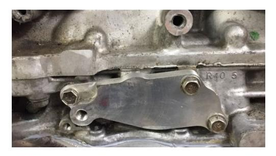
Next, flip the block upside down to prepare to install the oil pump pieces. First, locate this oil jet:
