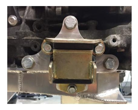
If replacement mounts are ever needed, use Energy Suspension part 3.1114G. One is needed per side.
