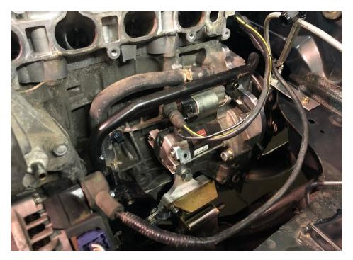
The black starter signal wire in our conversion harness has a "to starter relay" wire that allows you to use the factory K series routing. However, you can also just extend the Miata starter relay wire directly to the K series starter like we did in this picture and bypass the Honda harness and connector altogether.
