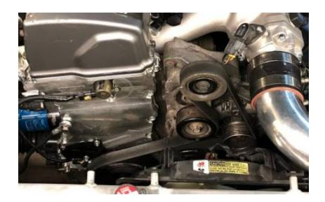
Any K series starter will work with this swap, although a starter that came from the same donor as your engine harness will make it a bit cleaner. You must use a 2009-2014 Acura TSX alternator, the older style K24 alternators do not fit on the K24Z3 water pump housing.
