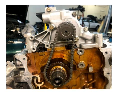
Use the supplied hardware to secure the pump but don't fully tighten the bolts yet.
