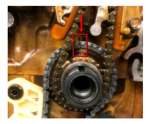
It can't be seen in this photo, but there is also a single gold link that corresponds to a mark on the bottom left side.
