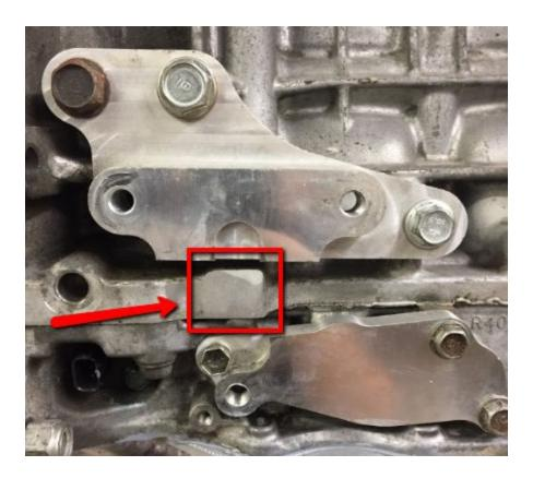
The Energy Suspension poly mount is installed on top of the bracket and oil filter block off, and it MUST be installed with the single backing plate that's supplied with your kit.
