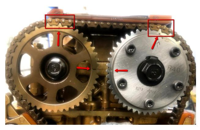
On the crank, make sure the gear is positioned at TDC and lined up with the arrow on the block here:
