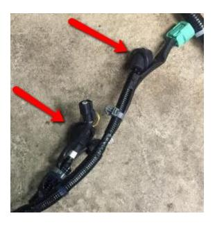
The green alternator connector is what needs to get replaced with a K24Z3 alternator connector.
