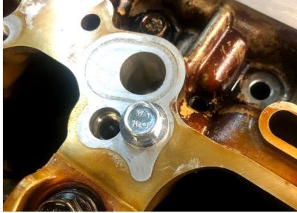
Next, you're going to install the small aluminum bracket that adapts the K20 pump to the K24Z3 block. These components are also included in the K24Z3 spec K20 oil pump upgrade kit:
