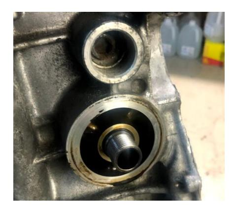
Your KMiata engine mount kit includes an oil filter mount block off and new OEM O-rings:
