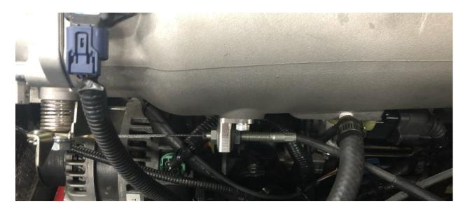
The supplied throttle cable bracket can also be installed. The throttle cable bracket provided is meant to work with an NB Miata cable. If you have any NA, you'll need to use an NB cable as the NA cables are very long and not suitable for this application. Cut the rubber grommet off the cable and clamp it in place tightly with the two 12mm nuts.
