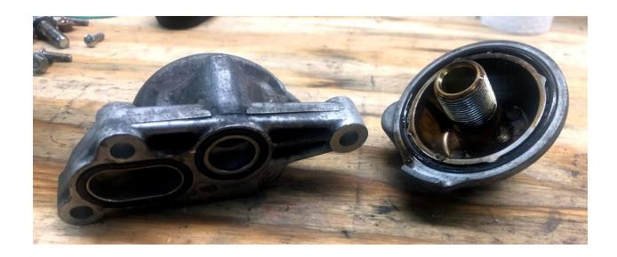
Your K20 oil pump upgrade kit from KMiata, specifically for the K24Z3, includes this threaded plug that allows you to install the oil filter in the older K series filter location on the side of the block. The Honda part number is 90015-PH1-013:
