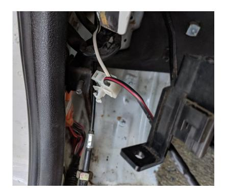
Alternatively, this black/red wire also pokes out to the engine back on the passenger side. This wire can be run directly to the K series starter and the black wire can be removed from the conversion harness altogether to bypass the Honda engine harness completely.
