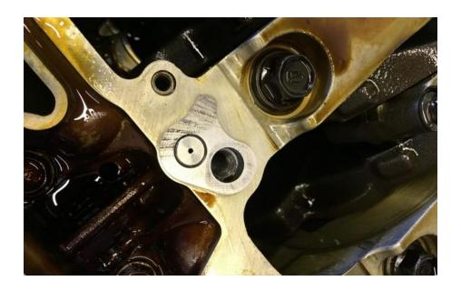
It NEEDS to be removed and plugged when installing a K20 pump. This is very important. You can either use a small drill bit to catch in the inside of the plug, or a small machine screw. Once it catches you can use pliers to pull it out.
