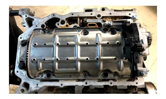
The pickup tube should be installed next, and then all bolts on the tray and pump can be tightened. Make sure the O-ring is present that goes between the pickup tube and oil pump adapter.
