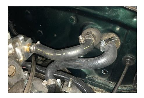
If you are not running heat, plug the upper port with the supplied ½" NPT plug, and we recommend the K-Tuned lower heater hose delete kit to plug the OEM plastic thermostat housing.
