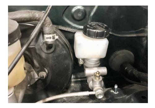
Take care to set the pedal height so there is a small amount of play before the pedal begins to push the master cylinder pin. If it is set too tightly, your clutch will not fully engage and it will overheat and slip.
