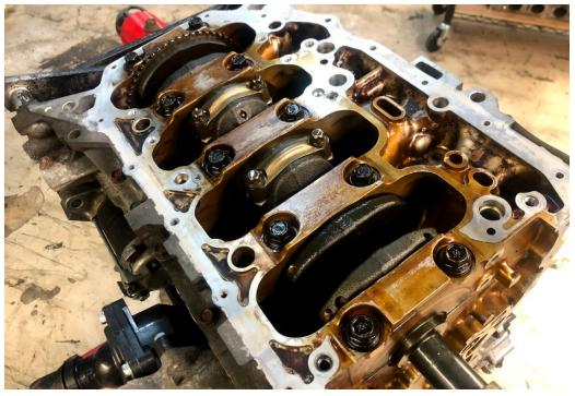
If you plan on re-using the tensioner, put a pin here before removing it from the block:
