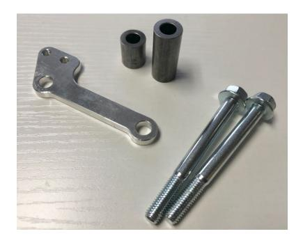
It's needed to support the leg that extends off the K20 pump:
