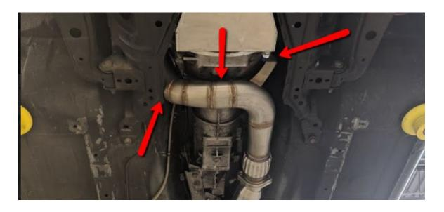
Additionally, six speed transmission users may need to grind down a bit of material directly above the oval crossover to avoid the downpipe rubbing on the bellhousing.
