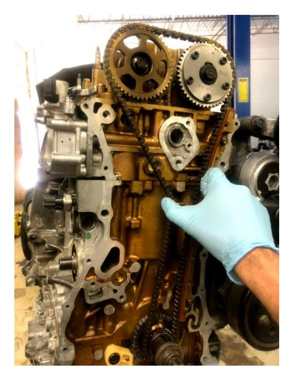
Once complete, the pin can be pulled out of the tensioner to lock everything in place. Use the crank pulley bolt and a 19mm wrench to spin the engine clockwise once or twice to make sure everything is turning smoothly.
