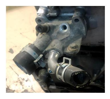
It needs to be replaced with the KMiata water neck. Reuse the K series engine coolant temp (ECT) sensor and thread it into the new water neck. The second port in the water neck is for the factory Miata temp sender to operate the stock coolant temp gauge:
