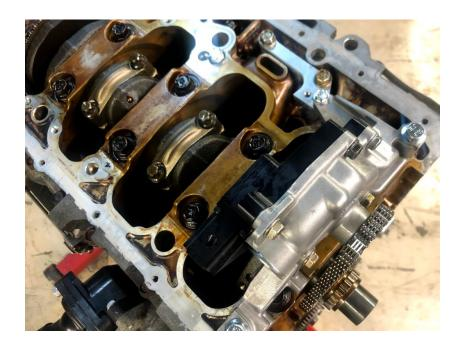
Next, the modified windage tray (also included in the K24Z3 oil pump kit) can be installed. The welded rails on the sides of the tray not only provide the correct mounting points to secure the tray, but also provide enough clearance for the larger K24Z3 rods that will hit the tray otherwise.
