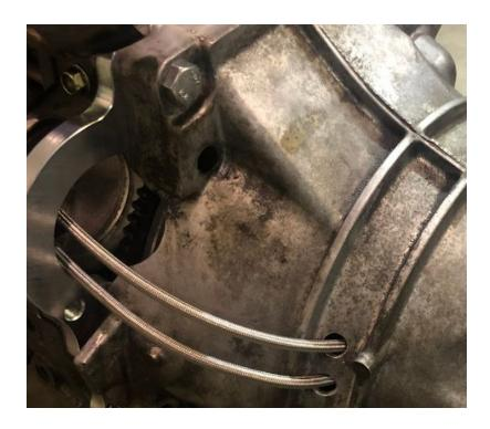
In order to provide 3 inch exhaust clearance on the right side of the transmission, our K24Z3 swap uses a custom hydraulic release bearing. This permits the factory Miata slave cylinder and clutch release fork to be deleted and allows us the space we need for exhaust routing.
