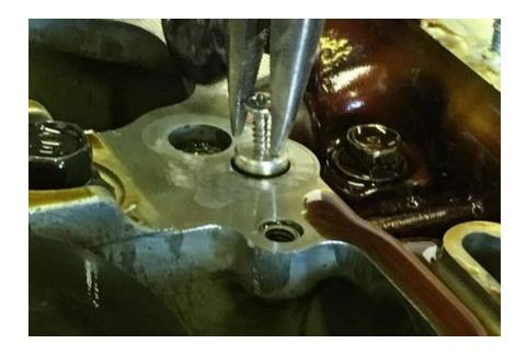
Your KMiata oil pump kit includes a short M8x1.25 bolt that needs to be threaded in to plug this hole. We also recommend putting a bit of Hondabond around the threads to ensure a perfect seal:
