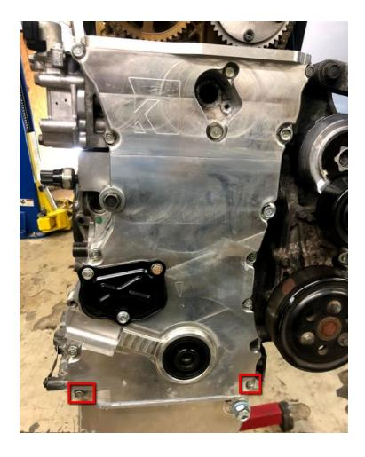
Note that the two lower corner bolts are the special bolts with the built in dowels:
