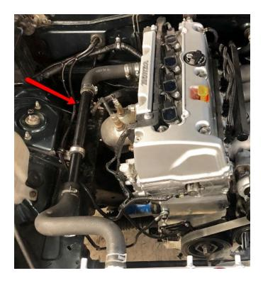
Finally, if you are running heat, you'll need to cut the lower heater pipe shorter and run a could %" heater hoses to the heater core, like this:
