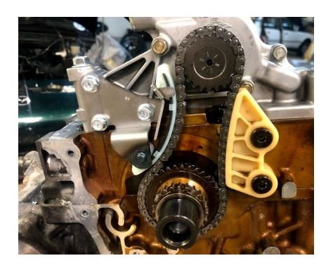
Next, the timing chain, guide, and tensioner can be re-installed.
