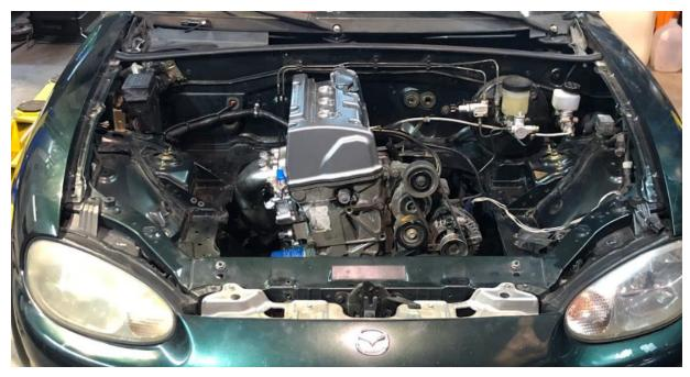
Note that on most NA Miatas and the occasional NB, the rear "shelf" in the engine may need to be trimmed by  $\frac{1}{2}$ " or so, otherwise the adapter plate will hit it:
