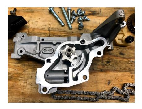
Our KMiata oil pump adapter replaces the stock pickup and provides the necessary pickup routing to clear your Miata steering rack:
