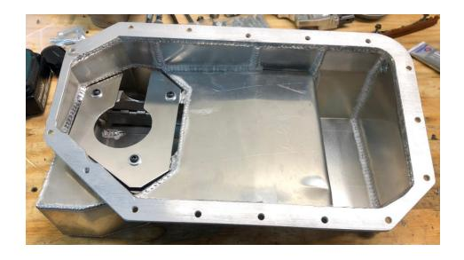
Carefully apply a bead of Hondabond directly to the bottom of the block *inside* the bolt holes for the oil pan.
