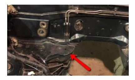
The Wilwood clutch master cylinder upgrade can be installed at this time too. Remove the Miata master cylinder and hard clutch line that crosses over to the passenger side of the vehicle. Both can be discarded.
