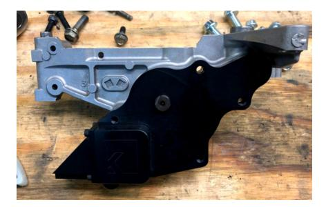
With the pump upside down in your hand, install the K20 oil pump chain (the K24 pump chain will not work) and hang the timing chain gear from it. Slide the gear over the crankshaft as you install the pump and line up the dowels:
