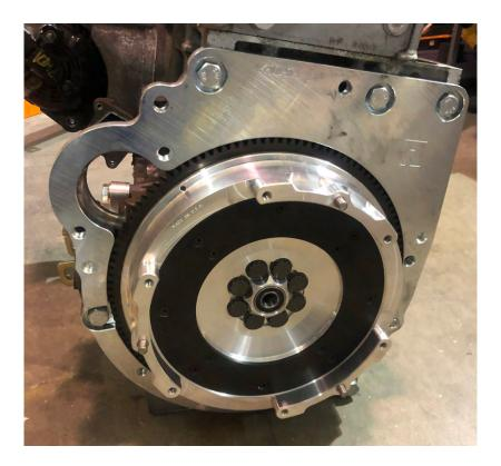
Note: If you are using an engine from a manual transmission donor car (rare), the engine dowel pins will be too long to fit inside the adapter plate. PLEASE do not just remove them, they are important to retain proper adapter plate fitment. You will need to replace them with the shorter 15mm dowel pins from an automatic car, Honda part **90701-PW5-000** (quantity 2).
