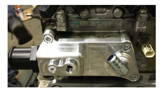
This piece includes three ports, from left to right:  $\frac{1}{6}$ " NPT port for an aftermarket temperature sender, a 12x1.5 port for your OEM Miata temperature sender, and a  $\frac{1}{2}$ " NPT port for a heater hose. Most builds will be configured as shown above, with the  $\frac{1}{6}$ " NPT port plugged, and the 90 degree barbed fitting pointed towards the heater core. Be sure to use teflon tape when installing the NPT fittings.
