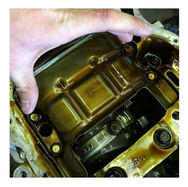
This small orifice needs to be removed and plugged in to our block. Use a wood screw to give it something to grab onto, and then pull it out. Alternatively, you can often remove it with a small, but sharp, drill bit. Start drilling into the center until the bit digs into the plug, and then pull it out on the bit. It's held in with an o-ring, so it shouldn't take a huge amount of force.
