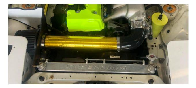
K series engines generally do best with at least 18" of intake piping, and the additional length also helps get the filter away from the hot engine bay. For street cars, positioning the filter inside the bay isn't as much of a problem, but a track car will heat soak pretty quickly and see intake air temperature spike with a short pipe and filter in the bay.
