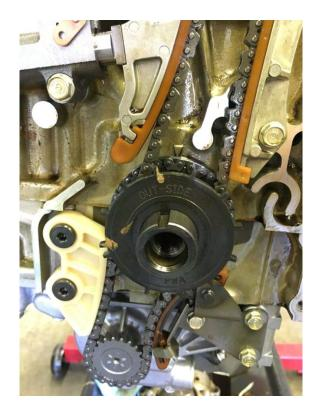
Now is a good time to perform any other valvetrain upgrades before timing the engine, installing the timing chain, and installing a brand new OEM chain tensioner if you desire.
