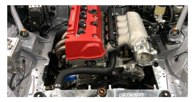
If you're retaining the stock auto tensioner and running the EPS idler pulley, you'll need a couple of longer hoses to route the upper hose around the belts and manifold.
