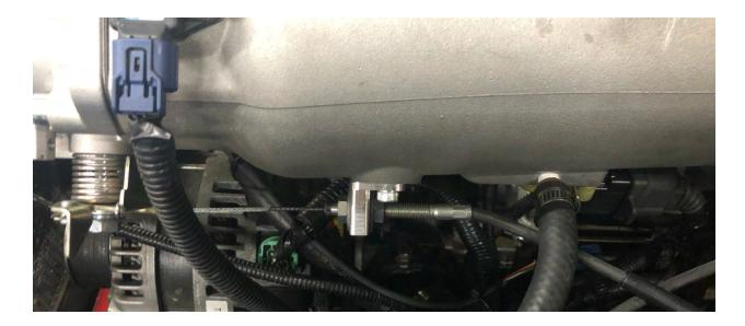
The supplied throttle cable bracket can also be installed. The throttle cable bracket provided is meant to work with an NB Miata cable. If you have any NA, you'll need to use an NB cable as the NA cables are very long and not suitable for this application. Cut the rubber grommet off the cable and clamp it in place tightly with the two 12mm nuts.
