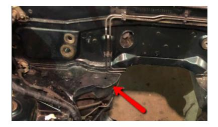
When bolting up the PPF to the transmission, be sure the tail end of the trans is lifted high enough, per the Mazda service manual. If the tail is too low you may experience drivetrain vibration, and your valve cover will also likely interfere with the hood.
