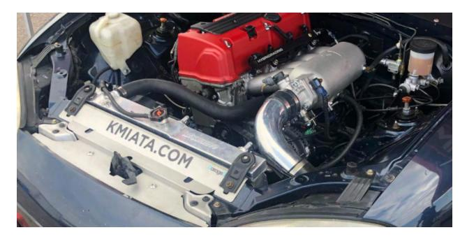
For a street car, it's less of an issue to keep the filter inside the engine bay with a simple setup like this:
