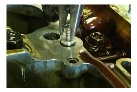
Once it's out, the block will have threads. Simply install a bolt to plug it. Our oil pump kit now includes this bolt (M8x1.25 thread pitch, with a socket head). Add some RTV on the threads to ensure a good seal.
