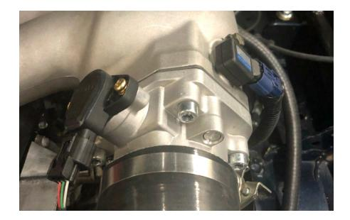
Note: We highly recommend against using the plastic "thermal" gaskets on the market, as they often cause manifold flanges to crack. An OEM style thin gasket is always preferred.
