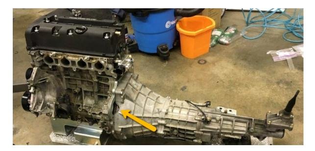
We used to do this modification with a reciprocating saw, but now we prefer to use a 2" hole saw for a clean, round cut. Here's a shot of the final profile. (Of course the clutch lines are in this shot temporarily and do not normally go through the starter hole).
