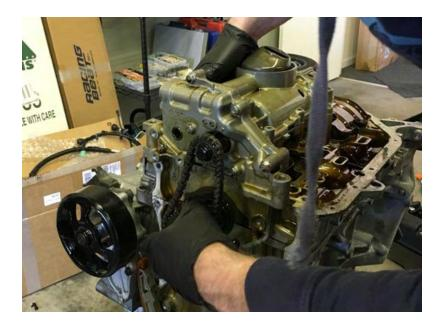
You will also use a new K20 windage tray to match the new K20 pump. Remove the OEM windage trays:
