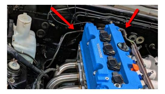
Additionally, AN fittings and lines can be used. Just cut the factory 5/16" hard line under the car, and use one of the -6 AN to hard line adapters on the market. We offer Hybrid Racing fuel rails that accept a -6 AN hose, and also allow a fuel pressure gauge to be installed on the rail.
