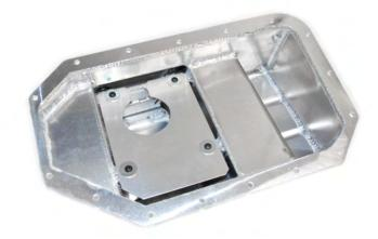
When you're ready to seal it, put a bead of Honda Ultra Flange or Permatex Ultra Black on the engine on the INSIDE and OUTSIDE of all of the bolt holes.
