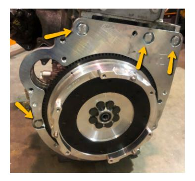
The remaining bolts secure the adapter plate through the engine side. One goes through the starter.
