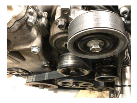
If you're running a car with no air conditioning, no power steering and the stock K24 crank pulley, use belt **7PK1320** along with the popular EP3 idler pulley setup.
