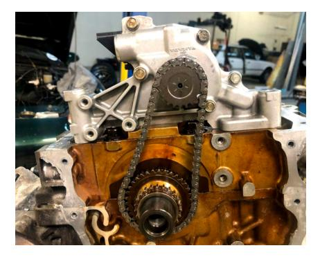
Use the supplied hardware to secure the pump.
