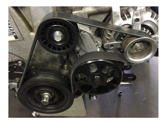
Note that there are some minor variations in size of these belts based on the manufacturer. We include 8mm washers, and you will likely need to use three of them to space the alternator out to give the belt adequate tension.
