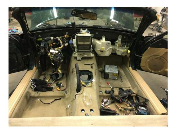
For race cars, all of the emissions-related components on the passenger side of the vehicle can be removed, as well as the vent line that runs from the charcoal canister back to the fuel tank (some customers may prefer to retain this). The only part that needs to remain is the larger fuel hard line, and NA Miatas will need to retain the return fuel line as well.
