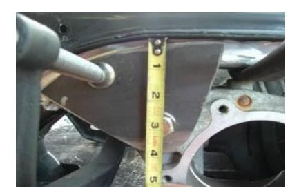
2. After locating the correct angle, clamp the plates in place and tack them to the subframe.
