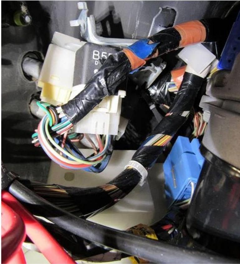
Step 5 - Before you mount the rest of the column assembly and motor, you will need to make room for it. There is a group of relays mounted on a small plate with 1 bolt hold it in place. Remove the nut and detach the plate from the bolt. Zip tie the out of the way towards the firewall or in whichever direction it needs to go to make room for the rest of the column. See the above picture for a general idea.
