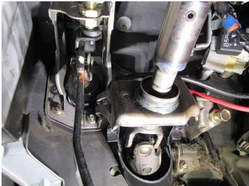
Step 3 – Loosen the set screws on the lower (short) steering shaft. Insert the lower steering shaft through the firewall mount. Insert the shaft into the u-joint. Put the bolt through the u-joint. The above picture show it assembled.
