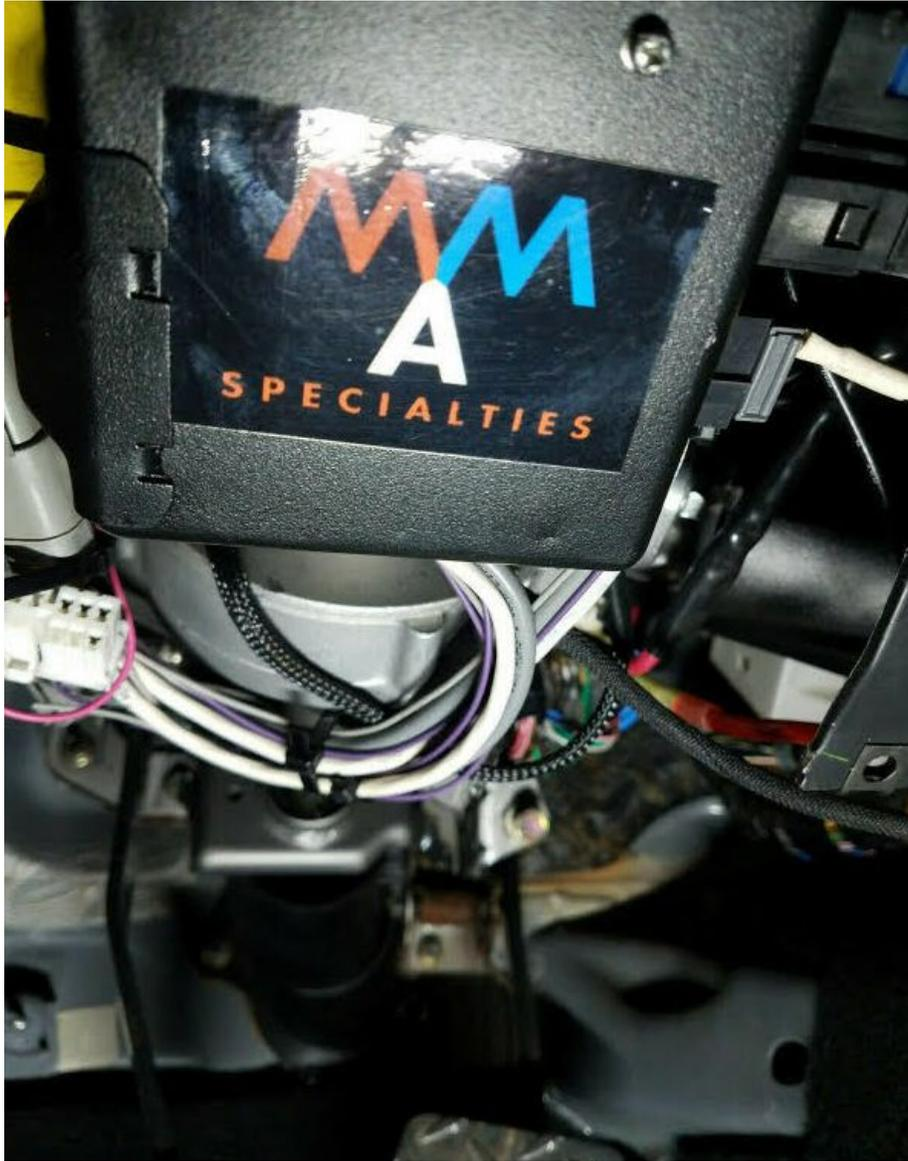
Step 4 - Connect the Power Steering assembly to the upper column assembly. The Electric motor will be facing to the right. Attach the ECU mount on the bottom bolt. See above picture except Do not install the ECU. This will be done later.
