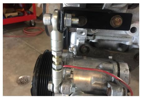
To install the belt, the tensioner should be turned to its shortest possible length. It may be easier to remove the upper tensioner bolt to slip the belt over the pulleys.
