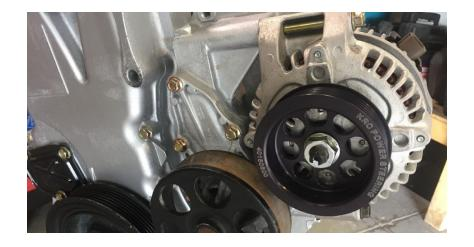
Next, remove the two lower alternator bolts to install the upper compressor bracket behind them:
