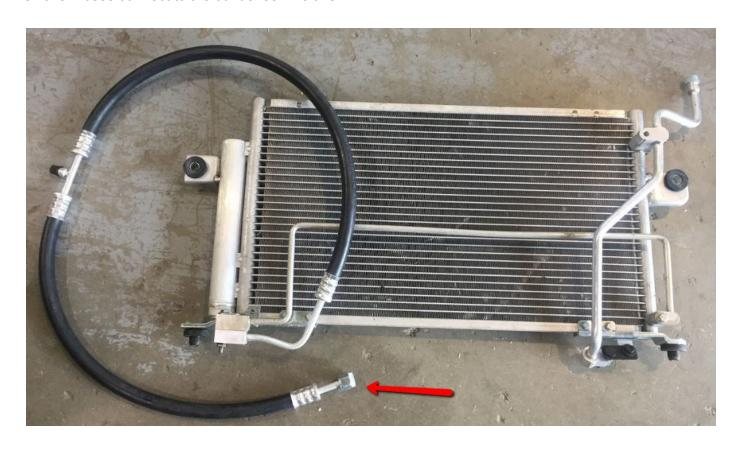
The #8 hose end indicated above runs along the passenger side frame rail and connects to the #8 port on the firewall.
