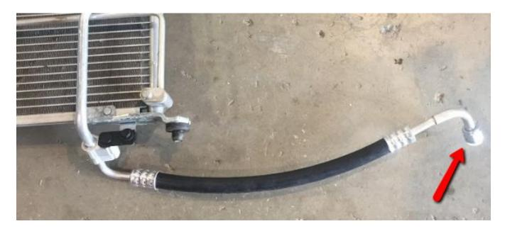
Use the supplied 10mm head nuts to bolt all of the aluminum fitting blocks onto the condenser.
