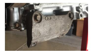
Using the supplied M8x1.25 bolts, attach the larger of the two steel brackets to the bottom of this mount:
