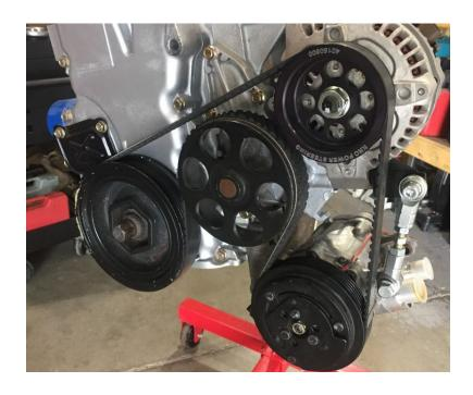
On the crank pulley, be sure that the 6 ribs closest to the timing chain cover are used so the belt is in proper alignment with the rest of the pulleys. The center 12mm nut in the tensioner can now be tightened to snug up the belt, and the outer 13mm RH and LH jam nuts can be tightened to lock the tensioner height in place. Don't forget to tighten the lower two compressor bolts once the tensioner is locked.
