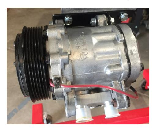
The tensioner can now be attached to the compressor and the upper steel bracket:
