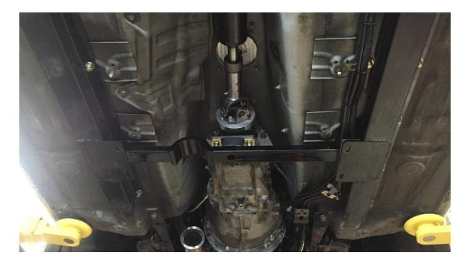
The supplied frame rails are installed just like any other frame rail on the market. The carpet must be removed and holes need to be drilled through the floor. Use the supplied grade 8 7/16" bolts, washers, fender washers, and nylon locking nuts to bolt the rails to the chassis.
