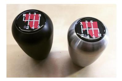
The KMiata knobs also include a set screw that can secure the shift knob at any desired height (this is why your shifter has a groove through the threads). We recommend using Loctite on the set screw to keep it from coming loose.
