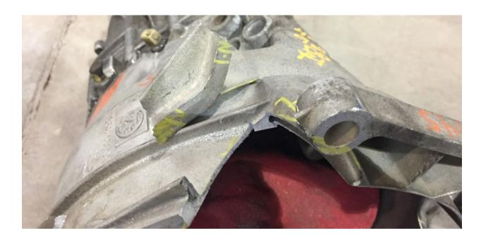
K series users have an easier cut to make. The K starter bolts directly to the engine, and only needs to protrude 3/4" into the bellhousing. Bolt the plate to the bellhousing and line up the starter, just as is done with the original K to Miata trans adapter.
