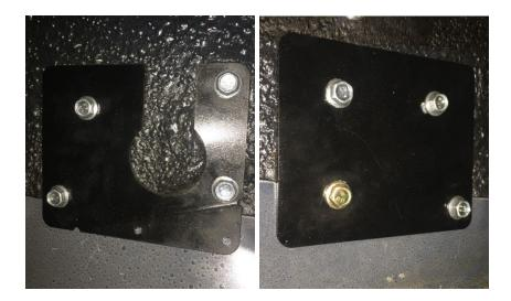
We supply the backing plates uncoated, as many racers will want to weld these plates to the tunnel to make service even easier. If you have no plans of welding them, you may want to hit them with some paint before installing.
