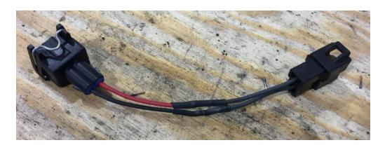
Now this jumper can be clipped into your Miata body harness and connected to the reverse light switch on the passenger side of the transmission.
