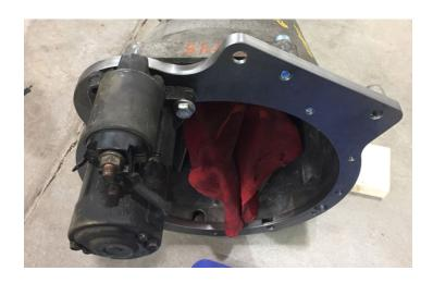
May 2018 Update: We recommend drilling out the threads on the Miata starter so it can easily be attached to the adapter plate. Note that there are variations in Miata starter bolt locations. Some starters will only line up with two bolts, while others will accept all three. Two bolts is sufficient and your starter functionality will not be compromised.
