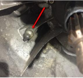
Once the release fork has been reinstalled with the retaining clip, install a new OEM release bearing. BP users installing a 5-speed will use the factory E46 release bearing included with any E46 clutch kit. K series to 5-speed users are required to install our custom extended stainless release bearing. Any user installing a ZF 6-speed (BP or K) will use the factory style release bearing. Note that it is not the same as the smaller diameter 5-speed bearing.
