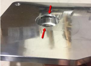
You'll probably need to flip the shifter and plate over and press the top of the shifter onto a hard surface to click the ball bushing tabs into place. It's meant to be very snug as you don't want any extra play in the shifter. The bottom of the plastic bushing gets compressed against the bottom of the shifter plate opening, so it will require a good amount of force to install. The groove in the threads on the shift lever should be facing away from the driver, towards the dash.
