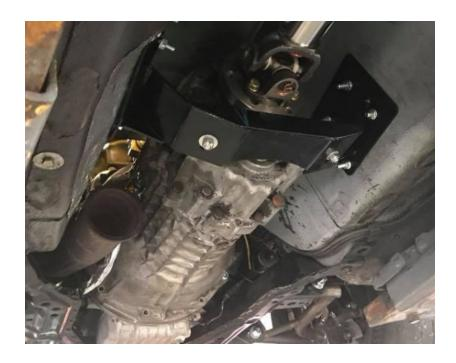
Since the PPF has been deleted, proper drivetrain geometry is important. On a stock Miata, the engine and trans slope back 1.5-2.0 degrees towards the rear of the car. *To double-check the transmission position, we recommend placing an angle finder along the transmission flange adapter. This should also be done on the differential to ensure proper drivetrain alignment. Both with a Getrag diff, and also with a Miata diff with a PPF delete.*
