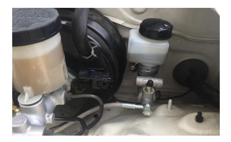
Once the factory master cylinder is removed, mock up the adapter against the firewall. You'll notice that some material on the firewall will need to be cut to fit the master fully into the opening. Use a Sharpie to mark the area that needs to be opened up, and use a Dremel or small cutting tool to shave away the excess metal.
