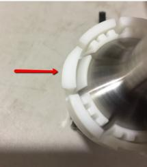
When the shifter and ball bushing are pressed into the shifter plate, those locking tabs need to be on the left and ride sides and are designed to click into the holes on the inside of the plate:
