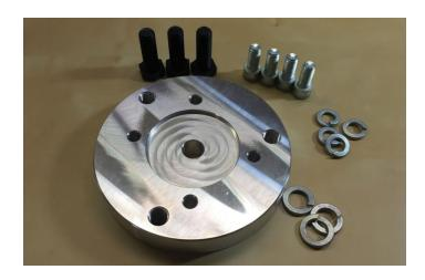
If you ordered your package for a Getrag differential, you have received two of these adapters. Although they look similar, the 3-bolt pattern is slightly wider for the differential. If you ordered your package for the Miata differential, no rear adapter is needed; we supply you with the correct flange directly on the drive shaft.
