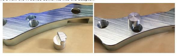
Once the OEM K dowel is pulled out of the driver side of the engine (below the starter), mock up the K dowel in the block. Before it is pressed it, line up the adapter plate so the D shaped end fits securely in the adapter. Once this is done, press the plate against the engine to seat the pin. If necessary, use a rubber mallet on the adapter plate to be sure the dowel is fully seated and the adapter plate sits flush against the block.
