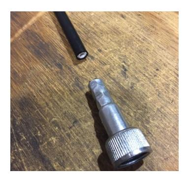
And cut the plastic fitting off the Miata cable and use some heat to fit it over the new cable. Position the end of the cable so it sticks out the same amount as the old cable end.
