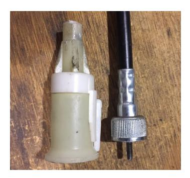
Cut the supplied cable to remove the fitting on the end:
