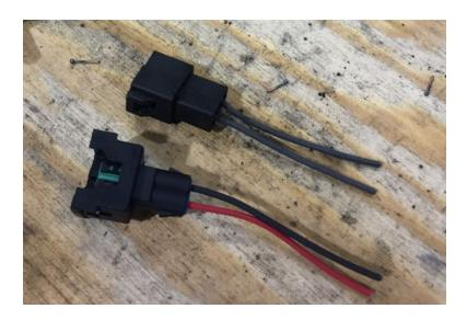
Solder the two sets of pigtails together and seal with heat shrink:
