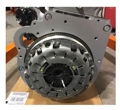
Note for Getrag 260 users: the E46 alignment tool won't fit inside the 12mm ID of the E30 style pilot bearing, and a regular E30 alignment tool doesn't have the removable shaft on the back to work with the E46 clutch. Because of this, you'll need to source an E30 alignment tool and do a little modification.
