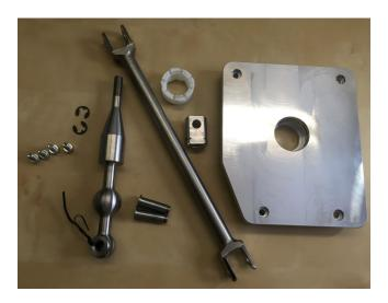
First, snap the shifter ball bushing onto the shift lever. We recommend greasing the ball before installing. Note the two tabs on each side of the ball bushing:
