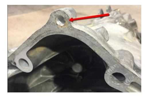
Next, inspect the parts inside the bellhousing. It's okay to reuse the shifter fork. Make sure the wire retaining clip is present, and also inspect the plastic pivot pin. These pins are a couple dollars and it's a good time to replace them. They can be pressed out from the outside of the bellhousing. Some BMW performance parts companies also make a stainless steel version that will never break.
