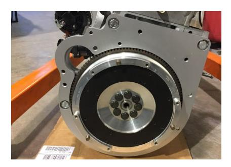
Both K and BP flywheels accept a BMW E46 OEM style clutch kit. If using a ZF 5-speed or Getrag 260, a clutch from an E46 5-speed 328i or 330i must be used. The disc has a 10-spline center, and the disc diameter is 240mm. The 228mm clutch kits from the 325i will not work, nor will the E46 M3 clutch. If using a 6-speed, the 22-spline clutch must be used from the 2003.5-2006 330i or 330Ci.
