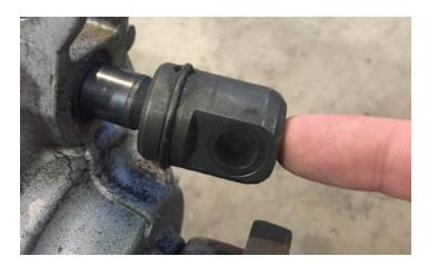
Getrag 260 users will notice that their selector joint is of a completely different design, with a different style retaining clip. As a courtesy we now include the E36/E46 style clip to make installation easy.
