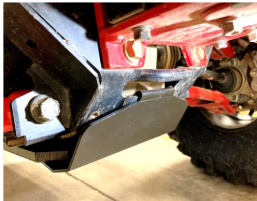
Bash Plate attached to Sheetmetal
