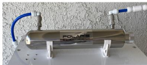
Connection Tube Installed
