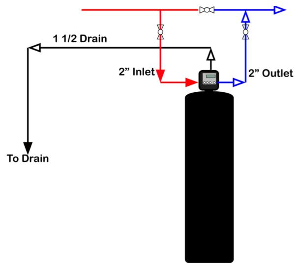
2" x 5 cf Cat Carbon System Connections Height 82" Tank Size 21" x 62"
