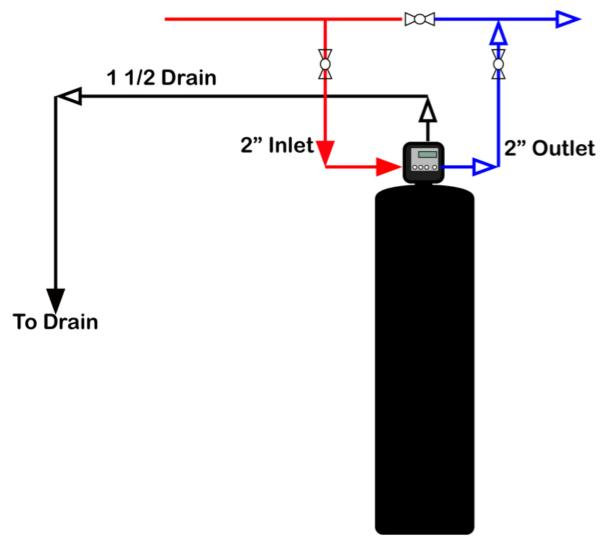
2" x 5 cf Cat Carbon System Connections Height 82" Tank Size 18" x 65"
