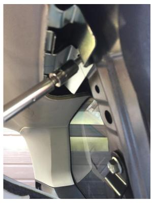
**Step 5**Align the above removed 10mm bolt to the supplied hardware as shown.
