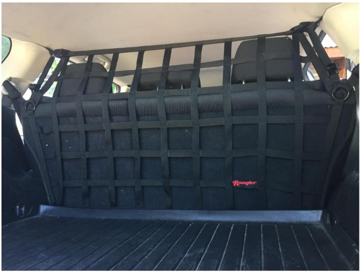
Position seat back into desired position and tension floors straps and then finally side middle straps. Pay attention that no obstructions occur with the seat back, the seat belts or any other trim pieces. Readjust if needed and finally wrap and tuck up the remaining strap ends.
