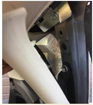
2015 – newer do not have the 10mm bolt. Install the footman C100 metal piece with 5/64" pilot holes above the round hole in approximate location shown. Proceed to **STEP 7**.
