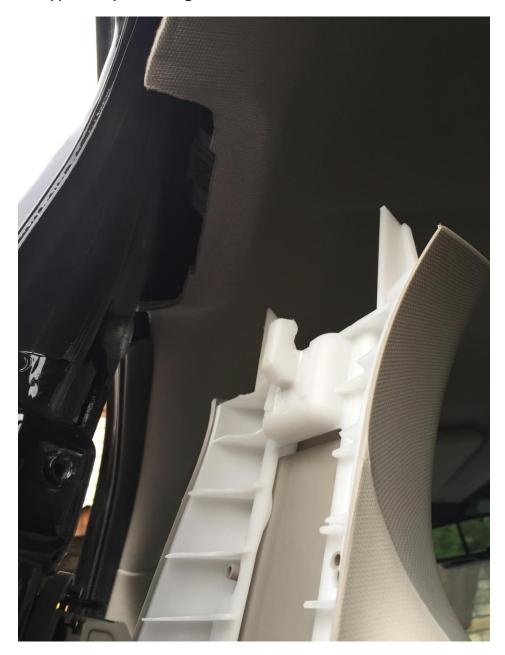
**Step 4:** Mount the footman strap by locating a good open metal surface as to not be too low to push down on the re-assembled plastic trim and not too high to interfere with the headliner material. Mark location on holes and pre-drill the mounting screws again being careful to check that no lines, wiring or seat belt interference will occur when re-assembled.
