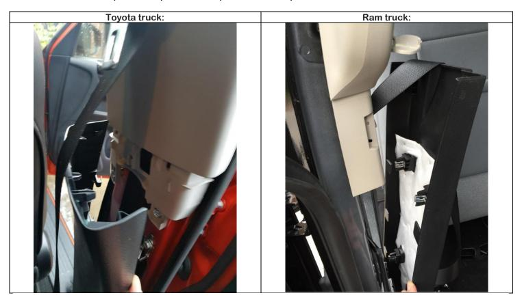
Be sure to look for fasteners in handle cover pop-outs and upper seat belt anchor bolts like the Torx bolt
