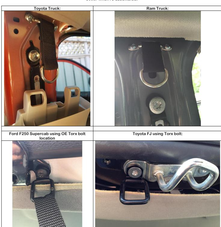
**Step 5:** Reassemble and check to ensure there are no obstructions to upper seat belt adjustment or trim panel fasteners, etc.
