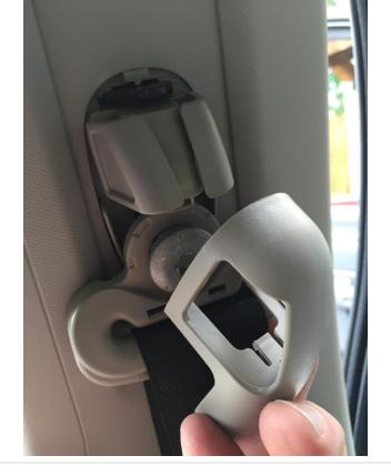
Step 3: Remove upper trim panel enough for access to the inner metal structure near the headliner
