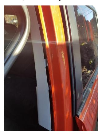
**Step 2.** This step is done similarly in most vehicles by loosening the upper part of the trim panel. Some vehicles this can be done by simply popping the trim snaps loose and carefully pulling out. Other vehicles may have a two-piece trim panel that requires the lower piece removed first as shown:
