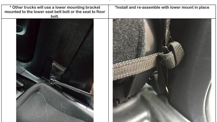
**Step 7:** Tighten the tension from top first, working your way to the floor. Pay attention to adjusting for normal seat positioning, wrap and tie off the excess adjusting straps.
