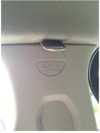
**NOTE:** the SRS stamp in the plastic is simply an identification marking and generally the actual SRS bags are in the overhead ceiling or in the seat themselves. Do look and verify that no plugs are unhooked, wires or actual components are damaged or altered.
