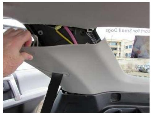
even upper seat belt pivot point bolts. In the 4Runner shown the rear passenger door rubber weatherstripping gasket was pulled loose at just the top back corner and by grasping the exposed plastic edge and the top above the 1/4 window glass, the panel pops loose easily. Be careful and be observant as to not damage the interior. Only the top edge needed to be loosened for access to install the mounts. IMG: 2010 - newer 4Runner
