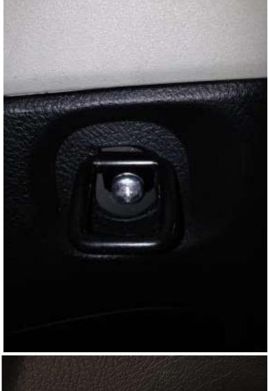
5th gen uses the rear wheel well mounted seat belt bolt for the lowest mounts. Remove the plastic cover and bolt to install the C101 chassis bracket as shown: (a full installation of the C101 set is available on our install documents page) IMG 5th gen 4Runner
