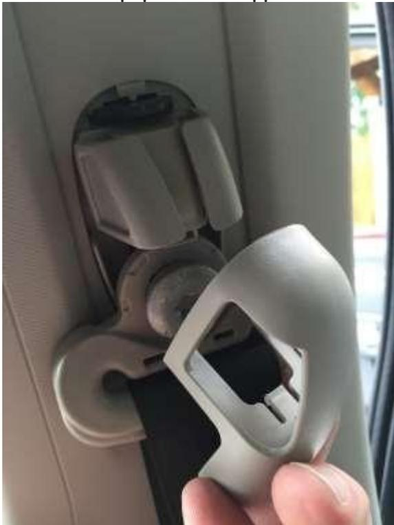
**Step 2:** Remove upper trim panel enough for access to the inner metal structure near the headliner
