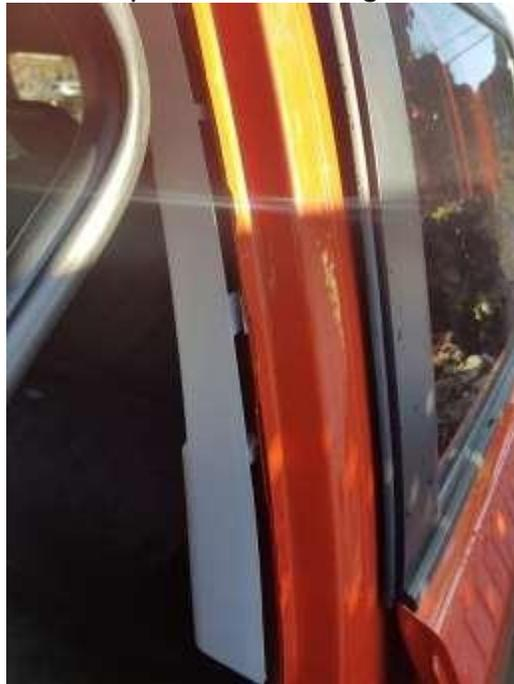
**Step 1:** This step is done similarly in most vehicles by loosening the upper part of the trim panel. Some vehicles this can be done by simply popping the trim snaps loose and carefully pulling out. Other vehicles may have a two-piece trim panel that requires the lower piece removed first as shown:
