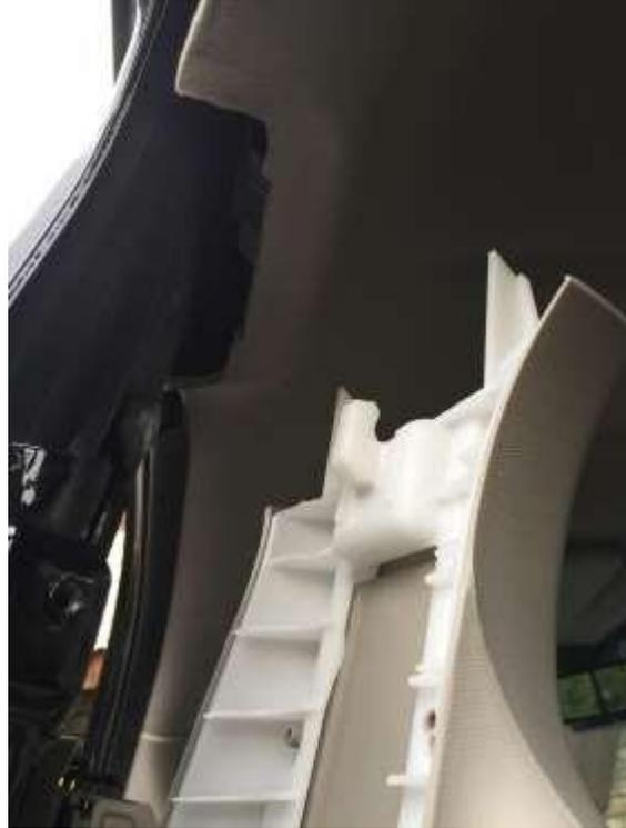
**Step 3:** Mount the footman strap by locating a good open metal surface as to not be too low to push down on the re-assembled plastic trim and not too high to interfere with the headliner material. Mark location on holes and pre-drill the mounting screws again being careful to check that no lines, wiring or seat belt interference will occur when re-assembled.
