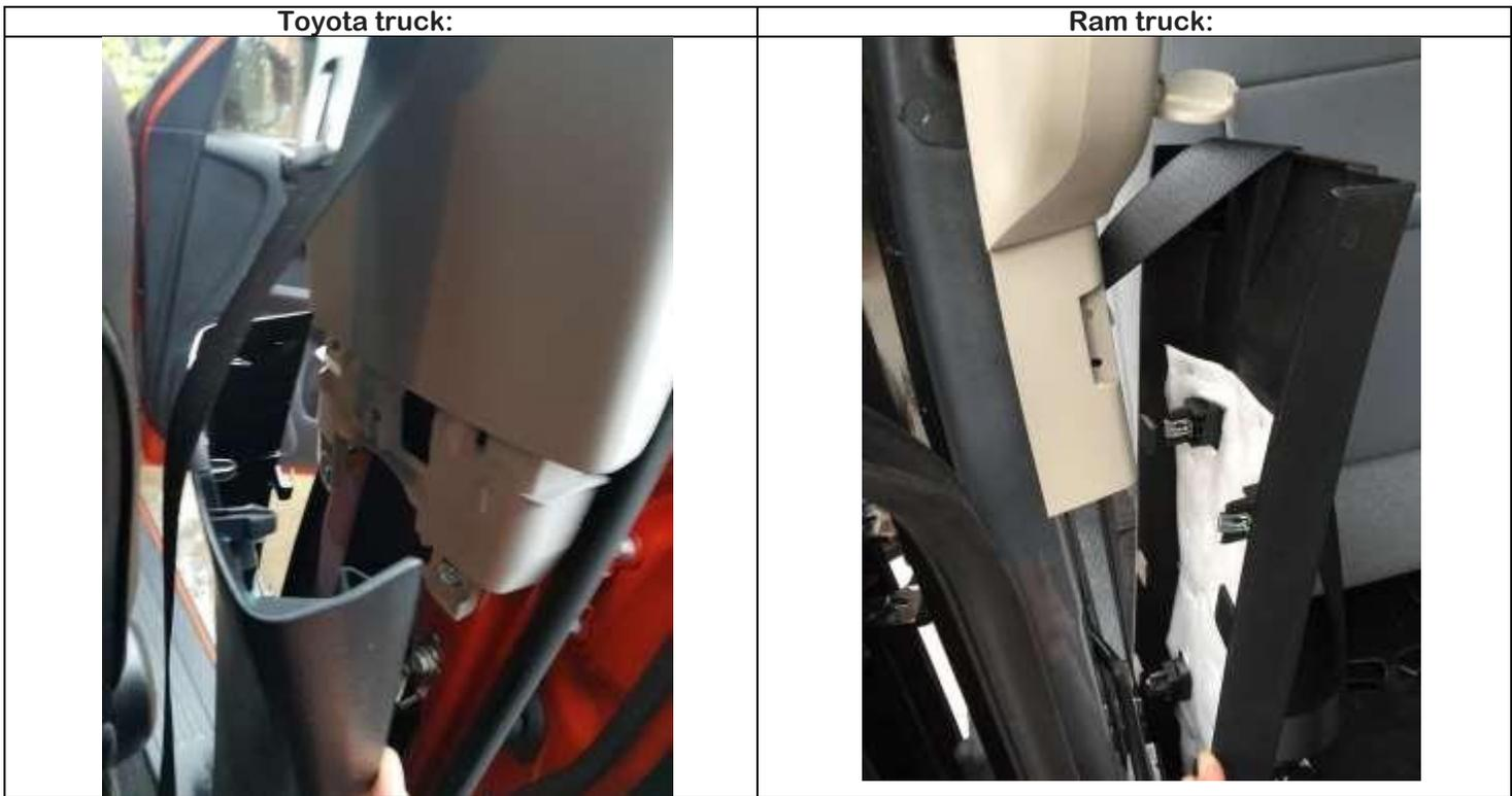
Be sure to look for fasteners in handle cover pop-outs and upper seat belt anchor bolts like the Torx bolt
