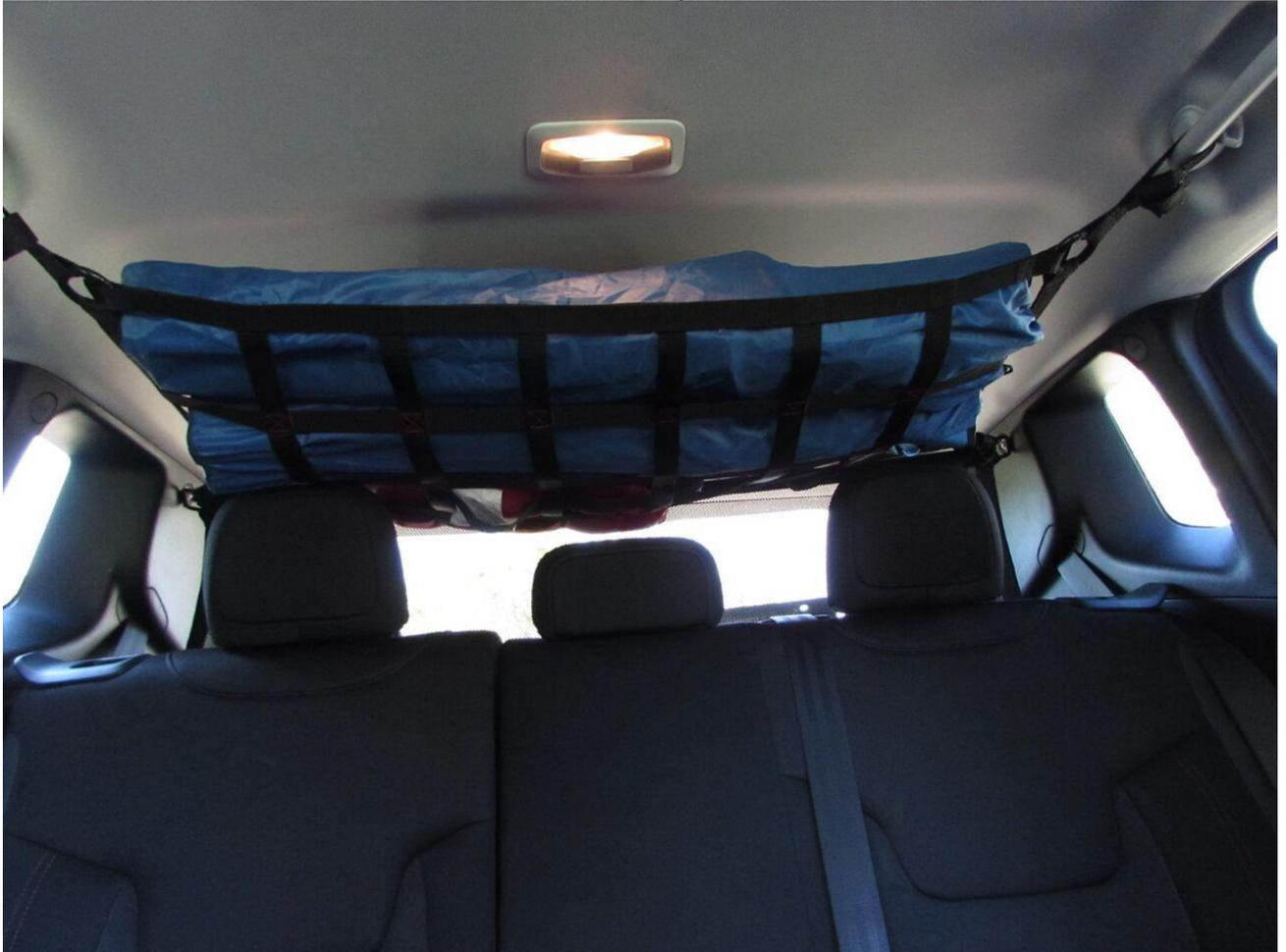
**Step 4:** Tuck excess strap back into buckle opening by the push tab, wrap around through the webbing loop on top of the push tab and tuck remained inside and pack into the loop. Enjoy your ceiling net. The rear barrier net uses the same mounts just installed and can be run in conjunction with the ceiling net. Also see our other Renegade products at [raingler.com](http://raingler.com)
