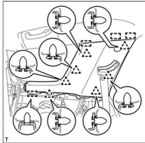
(b) Detach the 4 claws and 2 guides and pass the rear No. 1 seat outer belt floor anchor through the rear window side garnish assembly LH to remove the rear window side garnish assembly LH.
