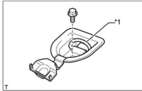
**31. REMOVE NO. 2 DECK BOARD SUB-ASSEMBLY (w/ Deck Board)**
