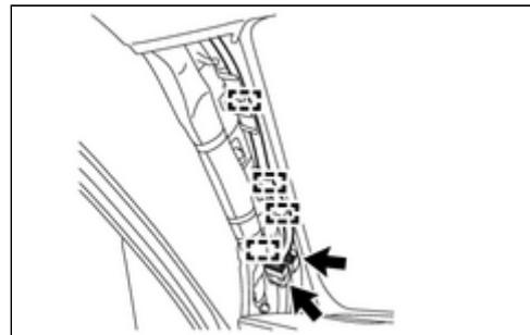
(d) Disconnect the connector and detach the 2 clamps from the front pillar RH.
