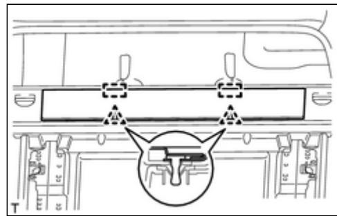
**32. REMOVE REAR NO. 2 FLOOR BOARD ASSEMBLY (w/ Deck Board)**
