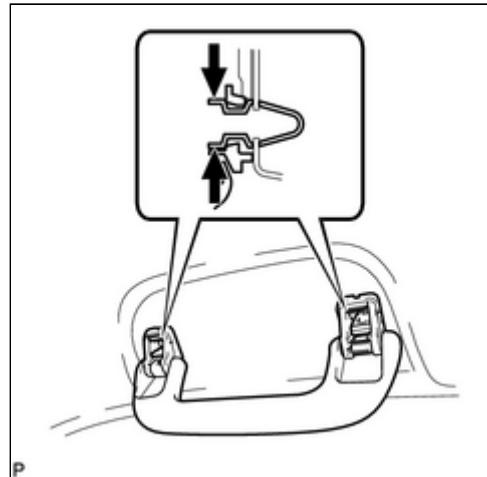
(d) Remove the 2 clips from the vehicle body.
