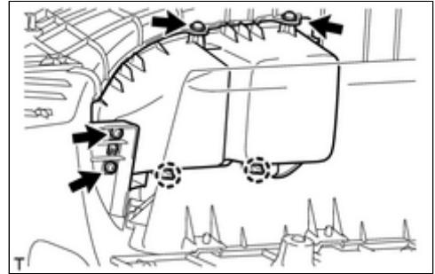
(b) Detach the 2 claws to remove the deck side trim cup holder LH.
