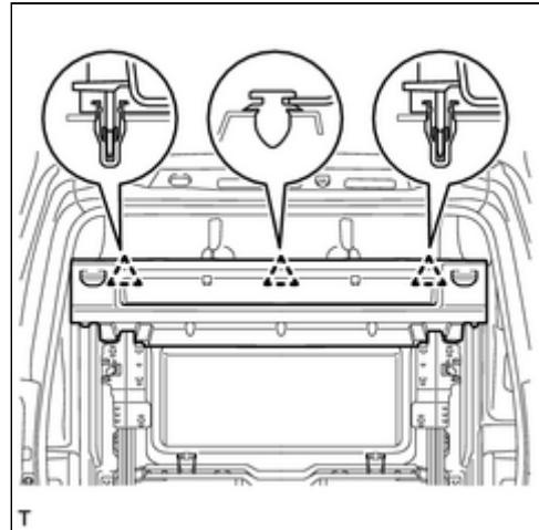
**33. REMOVE INNER FLOOR SIDE RAIL SUB-ASSEMBLY (w/ Deck Board)**
