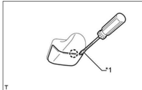
(b) Remove the screw and coat hook.
