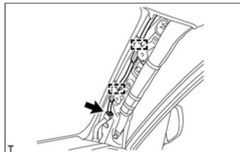
(e) Disconnect the connector and detach the clamp from the rear pillar RH.
