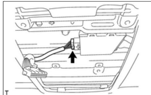
(c) Disconnect each connector and detach the 4 clamps from the front pillar LH.
