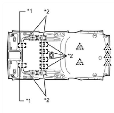
(h) Remove the roof headlining assembly from the back door as shown in the illustration.
