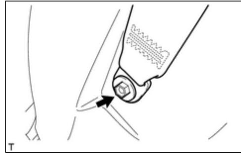
(2) Remove the bolt and disconnect the rear No. 2 seat outer belt floor anchor.
