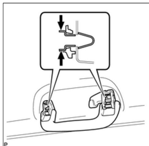
(c) Detach the 2 clips to remove the rear assist grip assembly.
