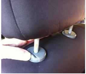
**Step 2**Remove headrest and slide handle onto pins
