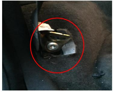
**Step 6**Install the top of the barrier and then the lower straps before tightening. Tighten straps - top first, then lower.
