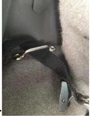
After all straps are fed through buckles, start by tightening from top to bottom and wrap and tuck excess strapfor a clean finished look.
