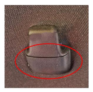
**Step 2.** Remove the OEM hook by releasing the spring clip with a flat blade or small needle nose pliers. BE CAREFUL not to let it get lost if it falls out of the hook. Carefully drill the pilot hole from the top side of the plastic hook once removed, and gently hand install the #12 screw holding down the grommet on the mount. Attach the hardware with the D-ring facing up, as shown.
