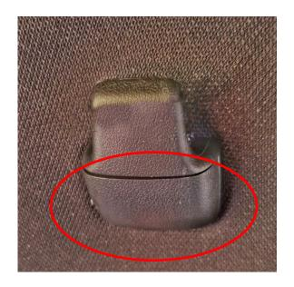
Step 2. Remove the OEM hook by releasing the spring clip with a flat blade or small needle nose pliers. BE CAREFUL not to let it get lost if it falls out of the hook. Carefully drill the pilot hole from the top side of the plastic hook once removed, and gently hand install the #12 screw holding down the grommet on the mount. Attach the hardware with the D-ring facing up, as
