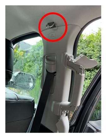
Barrier net installations will install the C119M bracket assembly under this lower seat belt Torx bolt next to the B pillar wall and angled up and back towards rear of cabin.
