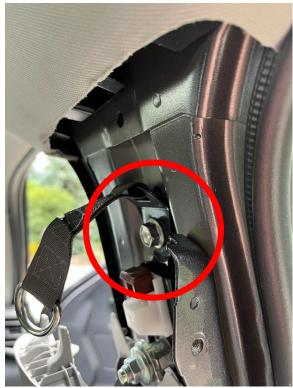
**Step 4**Feed the D ring and tether through the OEM opening BELOW the push in nylon tab:
