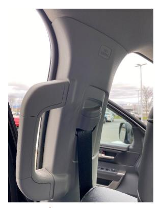
Gently squeeze to release the bolt covers on the B pillar handle. The trim panel removal tool may allow the cover to pop out and release if it's not easily done by hand. Note location of retaining leads as to not damage them during removal.
