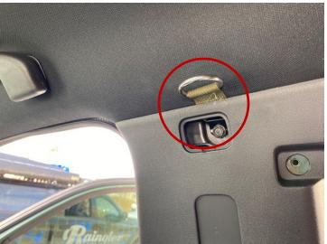
**Step 10**Reinstall handle bolts, covers and weatherstripping.
