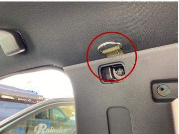
**Step 10**Reinstall handle bolts, covers and weatherstripping.
