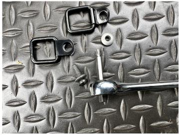
Stainless side of washer is next to the bolt's head. It's helpful to start installing the net from the top first but don't full tighten any straps yet. It's not critical which bolt is used on the back and top of speaker pod mounting bracket. We've used the one closest to the outside of the Bronco here.
