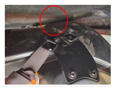
Hang the net now starting top to bottom. Feed the tapered strap end through the hardware points (or roll bar if installed that way) and back to the built on cambuckles. Depress the buckles tab and feed the strap end from underneath past the buckle's teeth. Then you can simply release the tab and pull taut. Do not fully tighten any buckles yet until the net is centered and at the proper height. The net should look something like this now:
