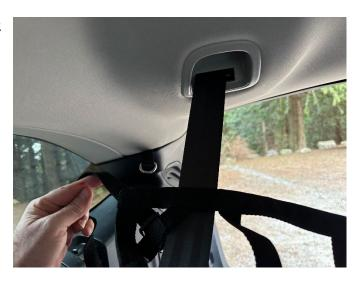
Squeeze tab on buckle and feed tapered strap end from bottom of buckle and through so the cambuckle's teeth hold the webbing. Do not fully tighten any straps until all are connected and the net is best centered side to side. The back of the net lines up just below the center overhead seat belt. A slight bit of touching is ok. Connect the next forward strap to the C pillar/side glass C100M D-ring and then the next to the 2nd row seat overhead handles:
