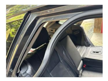
From the front top open edge grasp or use the panel removal tool to pull the trim back to release the nylon clips.
