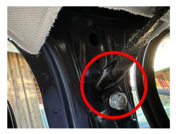
Install the hardware (Part C110XL) so the flat side of the tab is next to the inner B pillar and the tether and D-ring is oriented to the headliner. and reinstall the 14mm bolt.
