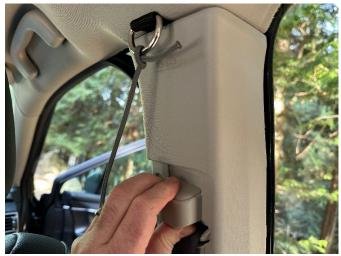
Reinstall the 10mm bolt in bottom of upper trim cover:
