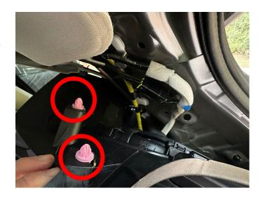
At rear of trim cover gently pry back enough to see and using panel removal tool, release nylon clip from hole (Driver's Side). Looking past the taped loom, you can see the second nylon clip:
