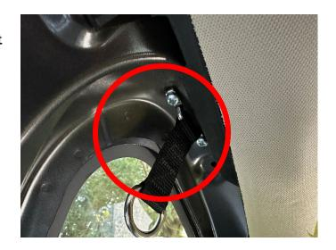
Check depth in area for mounting supplied #12 screws. Testing with a small punch in nylon clip hole by front corner glass:
