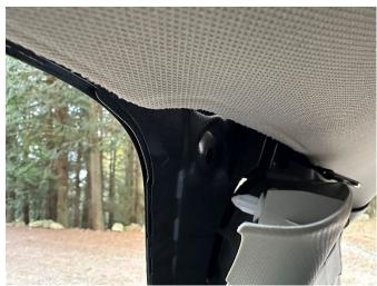
Once panel is full seated, line up weatherstripping and press back onto the C pillar ridge so it does not bunch and is neat and flat:
