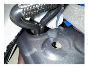
Install the hook of the C109R so that it catches inside the larger hole and orient the D-ring and tether towards the front of the cabin:
