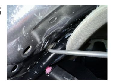
Pop the front edge of the trim loose at the headliner and down on the lower edge. There are plastic channels that the trim simply slides out of pretty easily:
