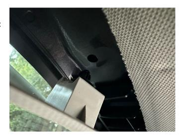
Watch that the nylon clips do not snag the headliner! Lace the shop towel above the nylon clips to protect the materials.
