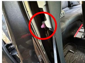
\*If this is not coming out easily, the upper panel can be slid up and then you can remove it and press into slot once panel has been removed in next step.
