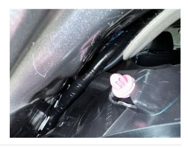
We find it easier to use a right angle awl to slide in and leverage the clip to release. Use care around the lines!
