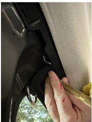
Punch a dimple in the location with a rubber hammer. TAKE EXTREME CARE that the hammer will not still and strike the window glass. You can drill the hole incrementally as shown in the preceding video until the drill can install the first screw. Do not use excessive force as to strip the screw or snap the screwed off.
