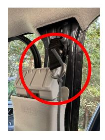
Feed the cord below the plastic piece the nylon clip mounts to and up through the openings between the outer upper trim piece as shown:
