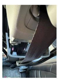
Press into place and press weather stripping evenly back onto the B pillar ridge:
