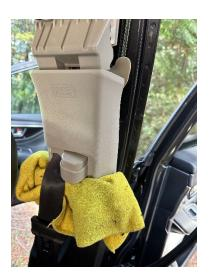
Detail of nylon clip above the upper seat belt 14mm bolt:
