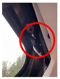
Step 12 Make sure that the D-ring stays clear of the trim panel while you reassemble the trim, lining up all of the nylon clips carefully before pushing back into the holes:
