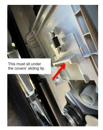
NOTE! Watch the upper seat belt mechanism (Printed "KNOB B PLR ADJ" beside vertical spring) BEFORE pressing trim cover back into place. The trim covers sliding mechanism must sit over the inner B pillar spring assembly (White plastic on left). Also the bolt must insert into the round short tube. Check that the adjuster works fully and that the nylon clip lines up to inner metal hole before pressing trim cover into place.
