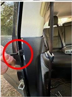
Once the side is loose, grasp the top edge and wiggle while pulling towards inside cabin to release the nylon clips shown below to expose the 10mm bolt at bottom of upper trim cover.
