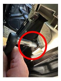
Looking in from the opening where the weatherstripping was, carefully pop the nylon clip on the lower portion of the upper trim with the panel tool from the front edge.
