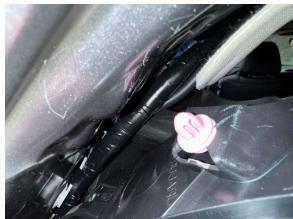
We find it easier to use a right angle awl to slide in and leverage the clip to release. Use care around the lines!
