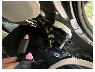
At rear of trim cover gently pry back enough to see and using panel removal tool release nylon clip from hole (Driver's Side). Looking past the taped loom, you can see the second nylon clip:
