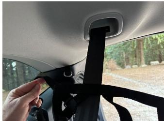
Squeeze tab on buckle and feed tapered strap end from bottom of buckle and through so the the cambuckle's teeth hold the webbing. Do not fully tighten any straps until all are connected and net is best centered side to side. The back of the net lines up just below the center overhead seat belt. A slight bit of touching is ok.
