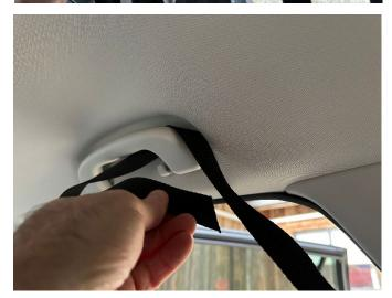
Start at the rear of the net and work forward to tension. The overhead seatbelt should not be restricted and access to the 2nd row seat grab handle straps should be in comfortable positions:
