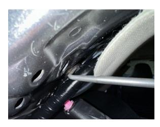
Pop the front edge of the trim loose at the headliner and down on the lower edge. There are plastic channels that the trim simply slides out of pretty easily:
