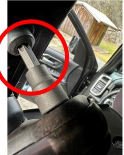
The lower Torx bolt will need to be loosened enough to allow the top of the bracket to come back off the B pillar enough to slide in the hardware piece.
