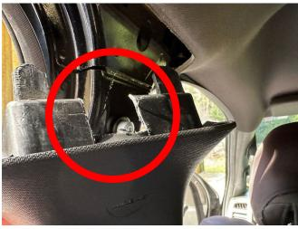
Step 5 Extract the upper seat belt bracket T-50 Torx bolt. Air ratchet works well as this bolt can be in there tight:
