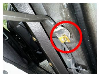
\*You will likely need to realign the anodized clips tabs so that they angle to slide back onto the plastic rides on the inside of the cover panels:
