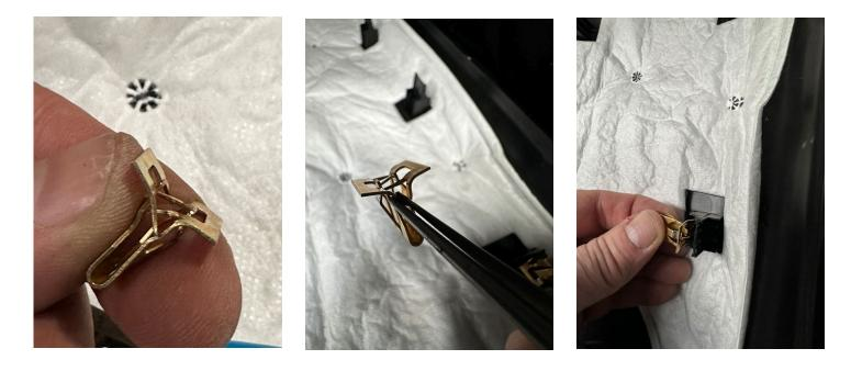
**IMPORTANT!** The top upper tabs must be reinserted into the slotted rectangular holes just under edge of headliner. You will have to watch that they stay in position while you keep the D ring over the top in the channel that was just made in step 4 and reposition the seat belt slider:
