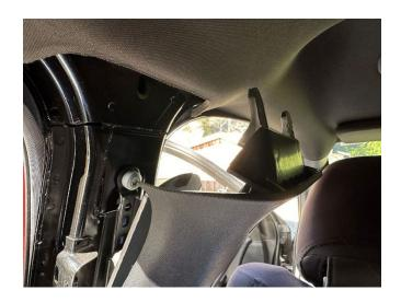
The flat plastic section between these two points will need to be trimmed down to allow tether access once the mounting hardware has been installed. It's hidden when reassembled so it doesn't have to be pretty or accurate. Just enough to allow 1" webbing to pass over this flat edge. Snips, Dremel or a hot cutter could all be used.
