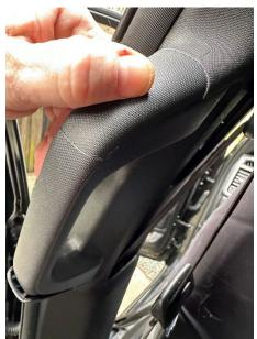
This is what the D ring and top of pillar should look like. If there is a gap at the top where the trim meets the headliner, double check that the two tabs are seated in their openings and the rubber weatherstripping is seated properly:
