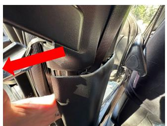
Loosen lower side edges of the upper trim in a similar fashion to the lower so that you can feel that it's loose. The upper seat belt adjuster can be raised and rotated to allow the upper trim piece to come off. It can also be removed and the belt slider bolt removed (not shown).
