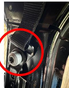
Reinstall any anodized clips that remained in the B pillar back into the trim covers:
