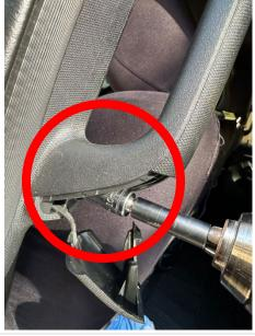
Grasp lower B pillar cover from back edge and wiggle and pull towards center of cabin. The rubber weatherstripping can be pulled up a bit for easier access.
