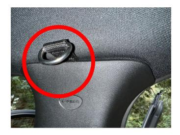
NOTE: It is easy to drop a screw, screw cover or the snap in nut down and into the cavity below. Go slow and take care not to do this. If this happens the rear seats will need to come out and while not hard will likely add another 30 minutes to the job and require the 18mm and E12 reverse Torx socket.
