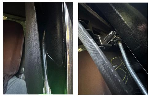
that you can see the cup that is behind the SRS marked pop out screw cover: Slide the awl from the front opening and insert through the side openings to twist and then pop out the screw cover.
