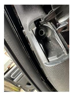
Reinstall the lower cover, paying attention that the seat belt webbing is not caught or restricted and can easily slide once panel is reinstalled.
