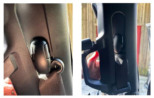
The top has two points that protrude into the upper B pillar openings just above edge of headliner. Wiggle and while pulling down, these will allow the whole upper piece to come off.
