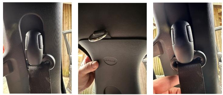
You will need to raise and lower the seat belt slider for best access. It's a bit tricky but patience and the second side will definitely be much easier once you've got this process down. The handle bolt holes should be perfectly able to align once everything, including the top tabs, are in place:
