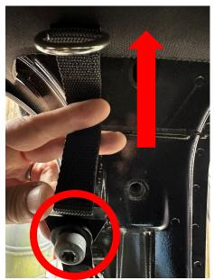
\*We have placed the bracket to the backside of the Torx bolt as to not require removal of the retainer nut.
