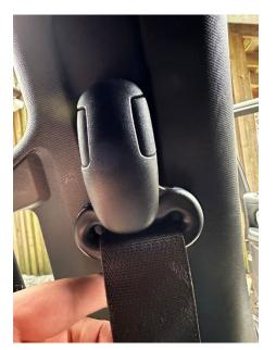
You will need to raise and lower the seat belt slider for best access. It's a bit tricky but patience and the second side will definitely be much easier once you've got this process down. The handle bolt holes should be perfectly able to align once everything, including the top tabs, are in place:
