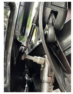
\*You will have to use care and slide the upper seat belt adjuster plate out of the way for access if not previously removed. Install the hardware piece C115XL with bracket angled in and tether and D ring oriented to top.
