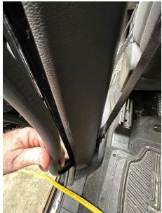
Double check that the upper seat belt slider can position up and down properly.
