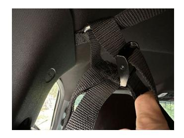
Do not fully tighten straps yet. Wrap next lower strap around the side B pillar handle and back into the buckles:
