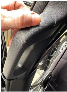
This is what the D ring and top of pillar should look like. If there is a gap at the top where the trim meets the headliner, double check that the two tabs are seated in their openings and the rubber weatherstripping is seated properly:
