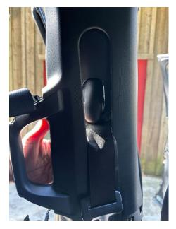
The top has two points that protrude into the upper B pillar openings just above edge of headliner. Wiggle and while pulling down, these will allow the whole upper piece to come off.
