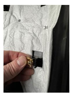
IMPORTANT! The top upper tabs must be reinserted into the slotted rectangular holes just under edge of headliner. You will have to watch that they stay in position while you keep the D ring over the top in the channel that was just made in step 4 and reposition the seat belt slider:
