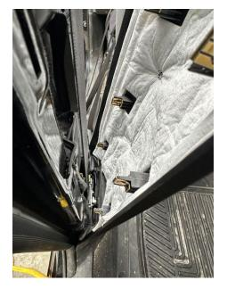
Reposition the rubber weatherstripping once both covers and all clips are seated properly:
