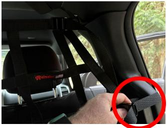
Feed the lower PVC coated hook onto the strap and hook strap end into buckle. Leave the loop long for now:
