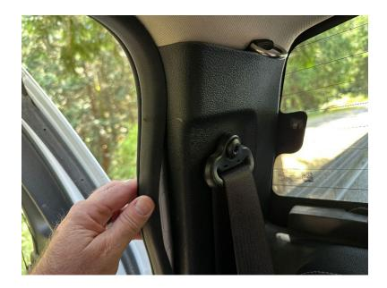
Reinstall T-50 Torx cover piece lower tabs and then press top into place.
