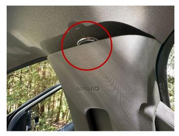
Double check clips are in line and the trim that goes under weatherstripping are properly lined up before pressing into place.
