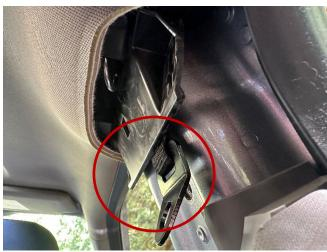
**Step 8**Line up bracket to seat belt bolt hole and reinstall with bracket next to inner B pillar structure.
