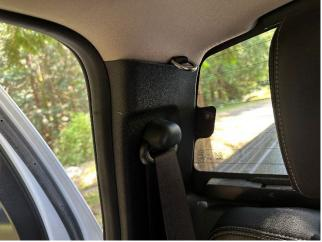
**Step 15**Loosely start to install the net starting at the OEM plastic hooks.
