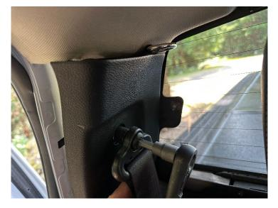
Check that panel is fully seated, headliner edge is behind trim fully and that the seat belt strap has free motion.
