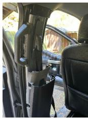
**Step 5**Slide the upper seat belt assembly all the way down.
