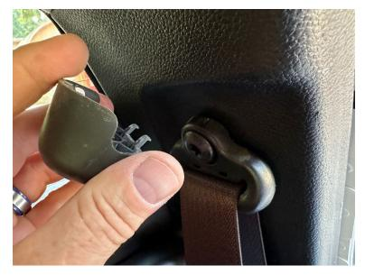
Used T-50 Torx wrench to remove the exposed bolt, taking care not to lose the retainer or collar on the bolt.
