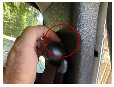
Tilt top back and lift up and out of two lower tabs.
