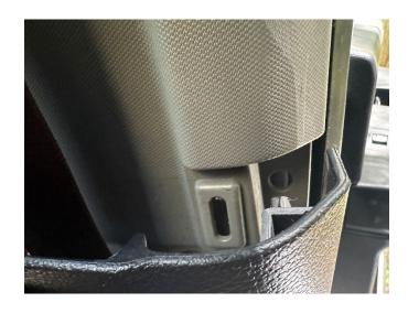
Use hand or panel tool make sure weatherstrip is on top of trim panel in both door openings. Be careful not to tear or cut the rubber.
