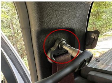
Set the seatbelt and bolt down out of the way for now.
