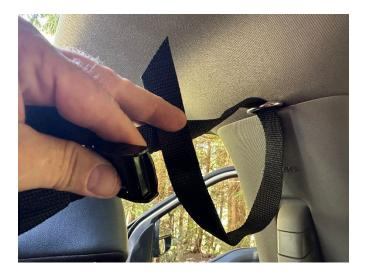
Run the tapered end of strap through the D ring and back to the buckle. Open buckle by pressing the tab to expose the teeth that will lock the webbing in tight.
