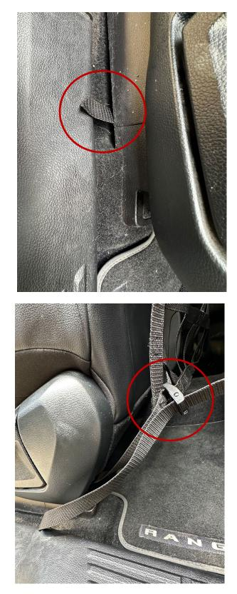
Hook strap end back to buckle at lower corner of net.
