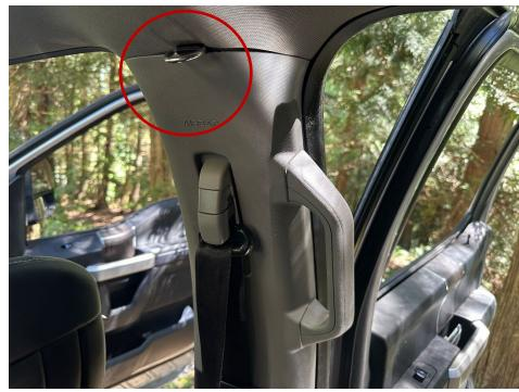
**Step 11** Start to install the net starting at the top to the D rings at top of B pillar.
