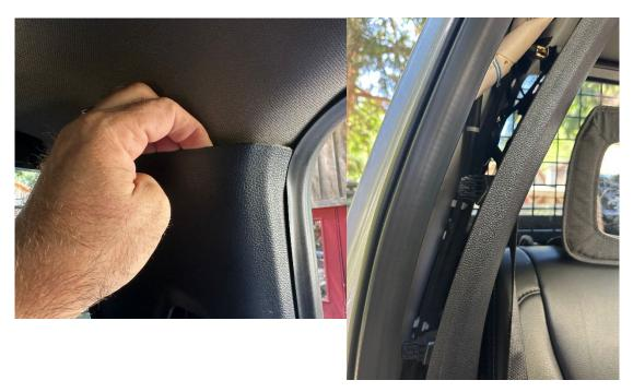
\*NOTE: Be careful not to lose the clips, and also make sure the anodized clips stay aligned correctly before reinstalling.
