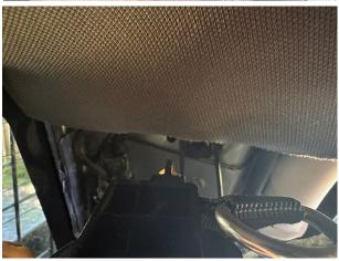
Be sure to keep D-ring above trim panel before fully reinstalling cover.
