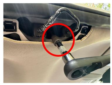
**Step 4**Reinstall the plastic cover with the D ring clear of the edge.
