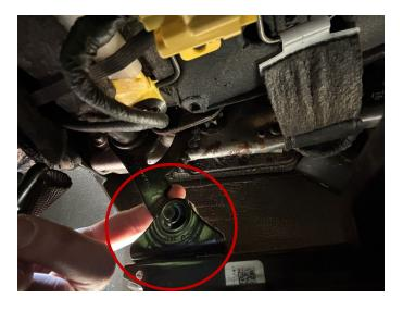
Place the hook in this notch. Snug up the strap just enough to keep the hook in place.
