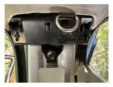
Reassemble upper panel, taking care to keep the stainless D-ring to outside of panel and also to make sure anodized clips are lined up to corresponding B pillar holes before pressing back into place.
