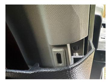
Use hand or panel tool make sure weatherstrip is on top of trim panel in both door openings. Be careful not to tear or cut the rubber.
