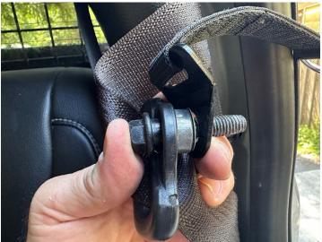
The webbing tether should route towards front of cab and clear of the anodized clip.
