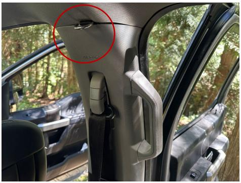
At rear of cab (C pillar) grasp top of trim cover and work back to pop top and side loose. This panel does not need to be fully removed.
