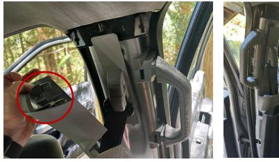
Slide the upper seat belt assembly all the way down.
