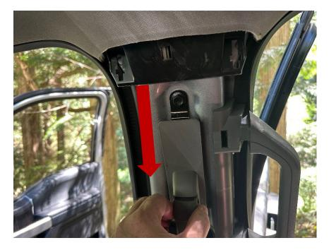
**Step 6** Using the 13mm wrench, remove the upper seat belt assembly bolt.
