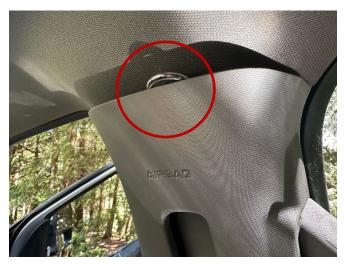
Double check clips are in line and the trim that goes under handle are properly lined up before pressing into place.
