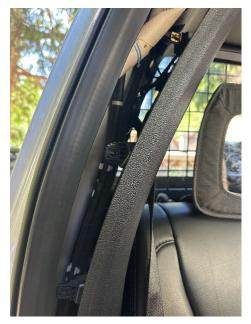
\*NOTE: Make sure the anodized clips stay aligned correctly before reinstalling and be careful not to lose them.
