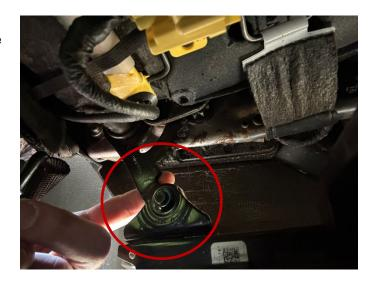
Place the hook in this notch. Snug up the strap just enough to keep the hook in place.
