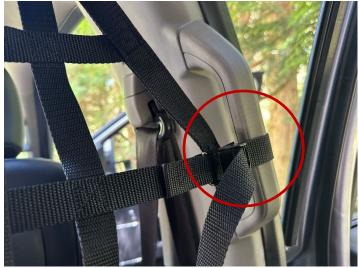
**Step 12**Install C109W hooks on lowest straps about 10 inches from corner of net.
