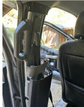
Slide the upper seat belt assembly all the way down.
