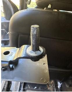
Install the C115L hardware piece with the angled end pointed to inside of cab and feed the D ring tether up just slightly towards rear of pillar to avoid plastic tab inside and under black piece.
