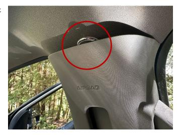
Double check clips are in line and the trim that goes under handle are properly lined up before pressing into place.
