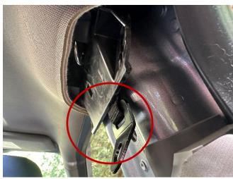
${\color{red} Step 8} \\ {\color{red} Line up bracket to seat belt bolt hole and reinstall with bracket next to inner B pillar structure.} \\$
