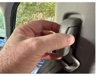
Squeeze the cam buckle and feed the strap end from underneath and up through the teeth and slot:
