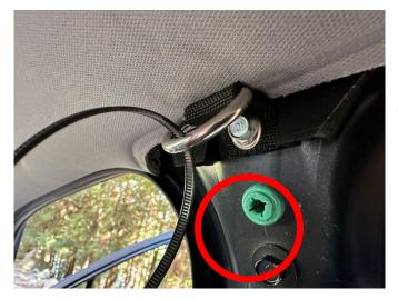
sliding down and off of the trim cover. You can then lift the side tabs of the green piece from the metal insert and reinstall the green receptor back into the B pillar opening hole:
