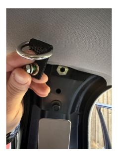
We suggest a large zip tie or string to make sure the D ring won't fall back into the panel during reassembly:
