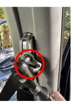
Remove the exposed 14mm bolt securing the upper seat belt adjuster:
