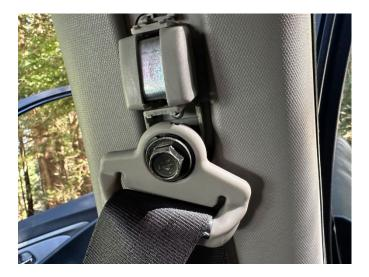
Ensure that there is no restriction with the seat belt webbing and reinstall the adjuster cover:
