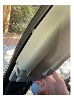
The service manual says that this clip should be considered a "one use" clip and to use a rubber mallet and a towel to tap it in, breaking off the protrusion tabs.
