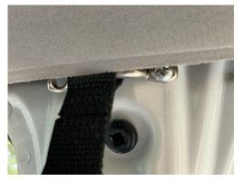
Since the holes are right at the edge of the flat part of the mounting surface, one screw was installed before punching and drilling second hole.
