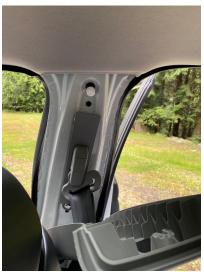
NOTE: The white plastic snap in is very difficult to remove and so we recommend a strong metal removal tool to pop it out. Reinstall this white insert back into the upper cover panel.
