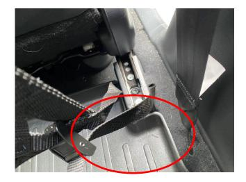
\*If you have the top quick release hooks you may have to adjust the tension so that you can lift the hook out of the pillar mounted C100S D ring.
