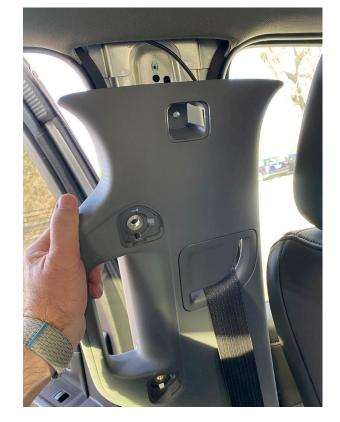
If your truck does not have this factory bolt, you may need to install one in this approximate location inside the round and slotted holes.
