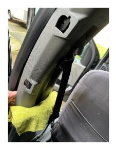
Rotate (either direction that's easier for clearance) the upper seat belt pivot to allow the unit to slide through the open channel \*(If not removed already in step 3)
