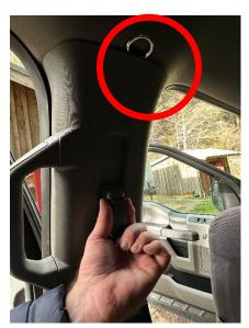
Check that weatherstripping is not stuck underneath the trim panels.
