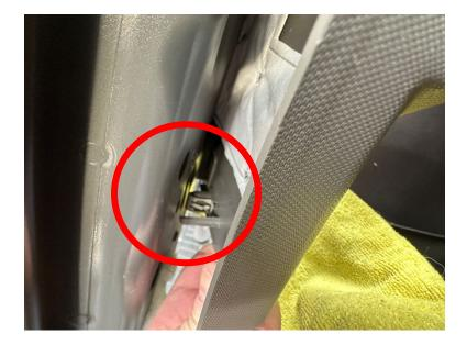
Check that seat belt operates smoothly and adjuster moves up and down as it should, free of obstruction.
