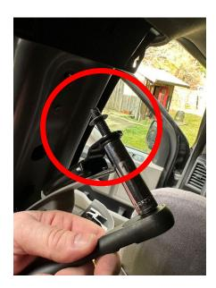
Push the nut back towards the bolt head if it's worked back onto the threads.
