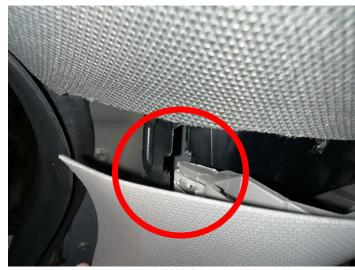
Line up lower panel tabs and press into position:
