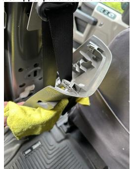
Step 7 Slide the Seat belt height adjuster down to expose the 13mm bolt under the plastic cover.
