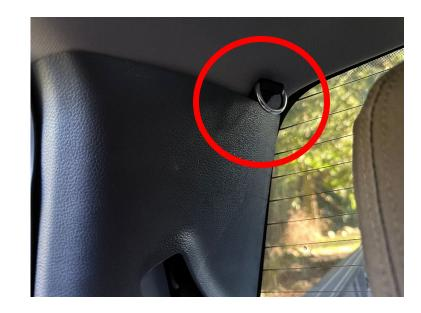
Double check that seat belts move freely and clear of any obstructions and press weatherstripping back into place.
