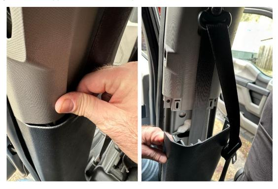
It may be easier to loosen the rubber weatherstripping just slightly to get ahold of the trim edge.
