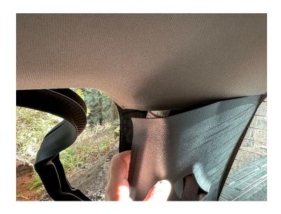
Many times these will easily pop off and out of the way. If you have a stubborn release clip and shown in the previous image (note the slight bend in the middle starting to form) You will need to use a pry bar that is included with most panel removal kits. You can access and barely see the brass colored metal clip from the front edge.
