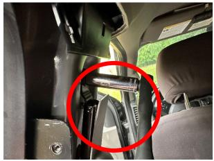
Watch to not drop or lose the retaining nut.
