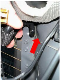
Step 14 Hold D ring out towards interior of the cab and line up metal clips and tabs to reinstall the trim cover.
