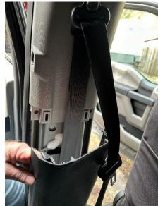
It may be easier to loosen the rubber weatherstripping just slightly to get ahold of the trim edge.
