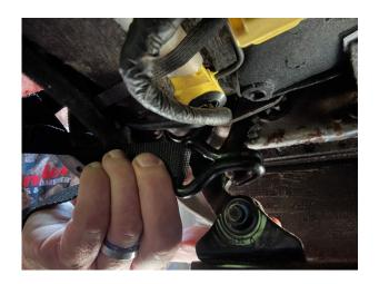
Lowest strap will feed forward to seat recline lever and route under the lever and through the opening at the rear outer side of the seating cushion. Reach under with other hand to feel for the tapered end of the strap and pull excess towards floor (shown on Driver's side).
