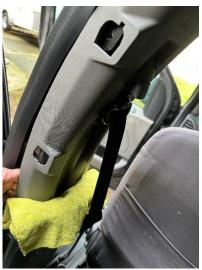
Rotate (either direction that's easier for clearance) the upper seat belt pivot to allow the unit to slide through the open channel \*(If not removed already in step 3)
