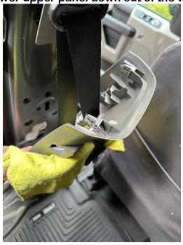
Step 7 Slide the Seat belt height adjuster down to expose the 13mm bolt under the plastic cover.
