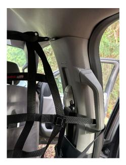
Depress tab on net's cam buckle and feed strap tip from backside of buckle up into the open slot's "teeth"
