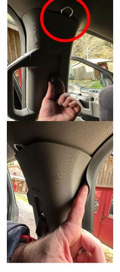
Step 10 Line up handle openings to bolt holes.
