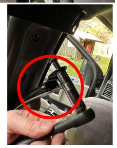
Push the nut back towards the bolt head if it's worked back onto the threads.
