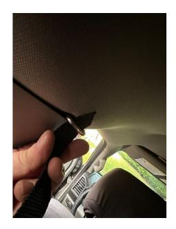
Do not fully tighten any straps yet. Feed middle side straps through handle on B pillar and back to the nets buckle.
