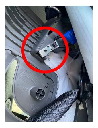
**Step 14** Slide the lower clip down and off the plastic edge:
