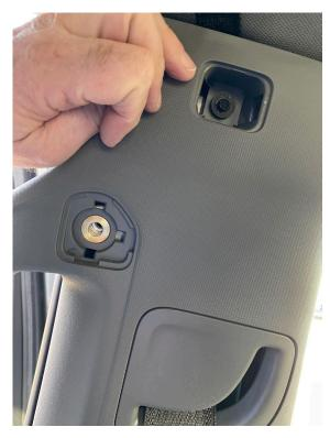
Tighten the 7mm bolt once assembly has been pressed into place:
