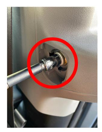
**Step 4** Top of side panel cover removes easiest from rear of cab
