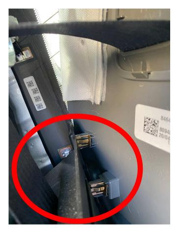
Note that there is a plastic tab that has to be lined up for the top to assemble properly. If necessary, loosen the C100X just slightly so that the tab can seat
