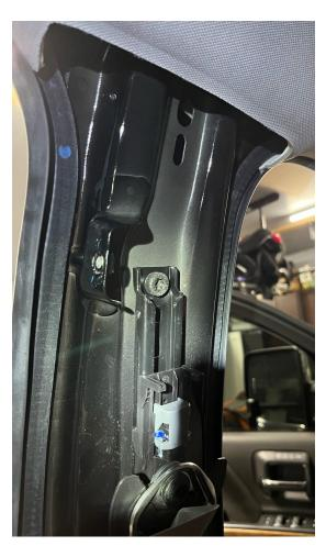
Slide the C100X hardware mount tab to the back side of the panel with the tether strap oriented to the top. The 7mm bolt removed in step 5 will slide into the C100X's mount tab hole
