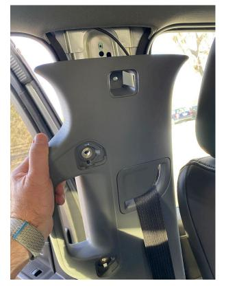
If your truck does not have this factory bolt, you may need to install one in this approximate location inside the round and slotted holes.
