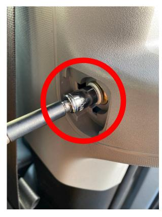
**Step 4**Top of side panel cover removes easiest from rear of cab
