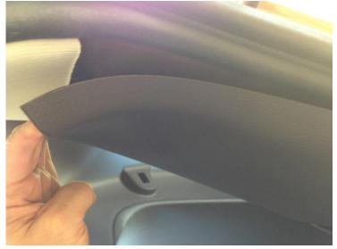
Step 2 Locate and note round hole and location of wiring harness on passenger side.
