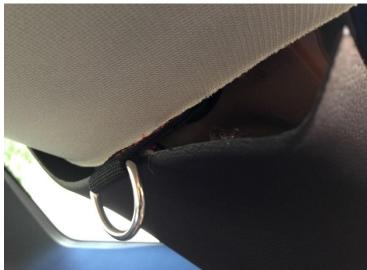
**Step 6**Carefully reassemble panels so that all OE snaps fit correctly into structure holes.
