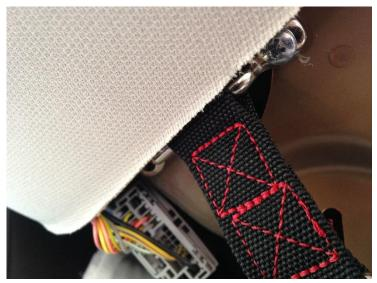
**Step 5**Re-assemble panel with D-ring extending out between panel and headliner.
